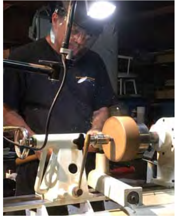
Attach blank with screw, round bowl out with roughing gouge.
