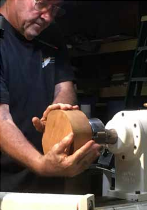
Attach blank with screw, round bowl out with roughing gouge.
