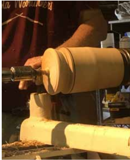
Smooth out and see how knots are arranged. Try to get knots to come across face
