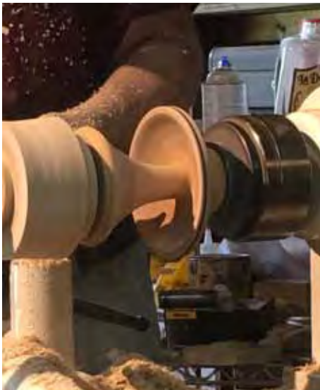
Use parting tool at base of mushroom. Drill and hollow out bottom so it won't crack.
