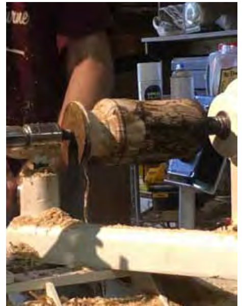
A second mushroom is begun. Smooth out with roughing gouge. Align knots as before.
