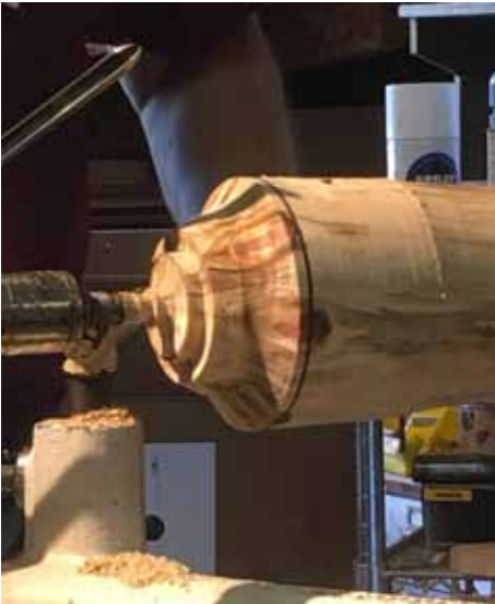
Make tenon. Use side of gouge on end grain to smooth out. Reverse piece on lathe, secure in chuck.
