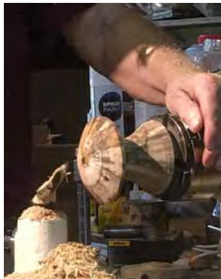
Shear cut top with flute pointing south. Norfolk Pine is full of sand so you'll sharpen tools more often.
