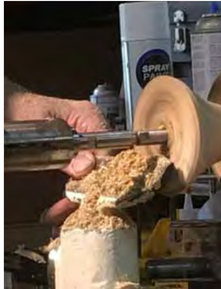
Drill base and then hollow with spindle or roughing gouge to keep from cracking.
