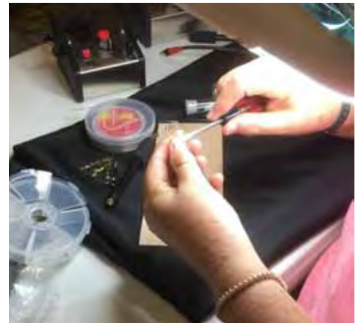
Various nibs can be easily made for different burn patterns.
