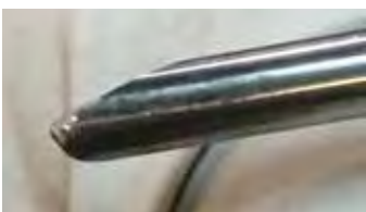
Steve's 60 degree gouge grind.
