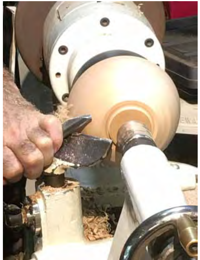
Downhill shear cut, elbows in, handle against hip, right foot in front.
