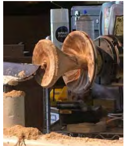
Use parting tool at base of mushroom. Drill and hollow out bottom so it won't crack.
