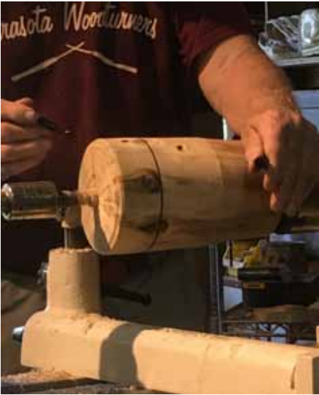
Smooth out and see how knots are arranged. Try to get knots to come across face
