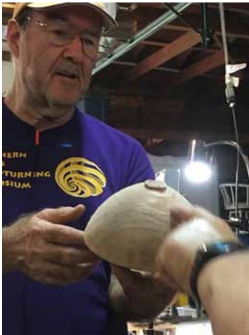
An interior cut out bowl. Use a tail stock extender to secure bowl at end of cutting.
