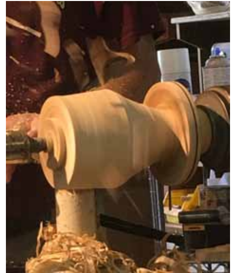
Make tenon. Use side of gouge on end grain to smooth out. Reverse piece on lathe, secure in chuck.
