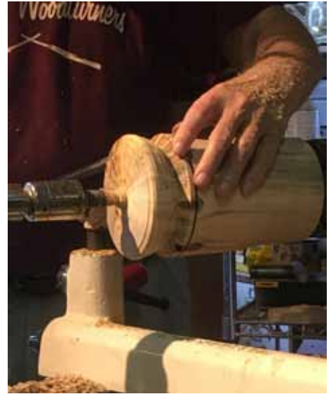
Smooth out and see how knots are arranged. Try to get knots to come across face
