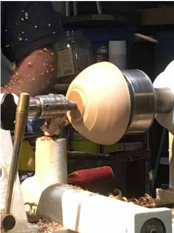
Downhill shear cut, elbows in, handle against hip, right foot in front.
