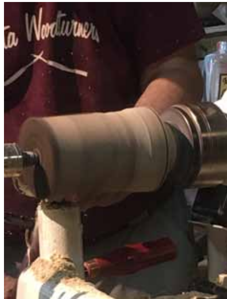
A second mushroom is begun. Smooth out with roughing gouge. Align knots as before.
