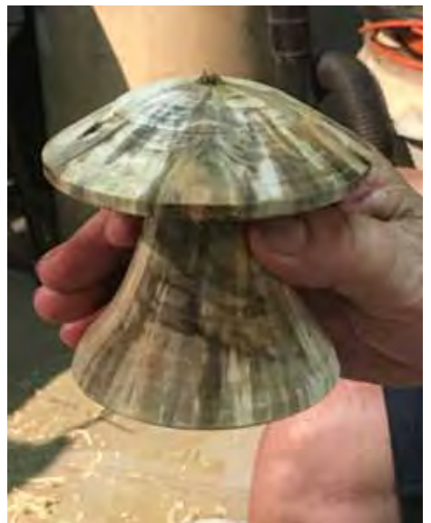
Shear cut top with flute pointing south. Norfolk Pine is full of sand so you'll sharpen tools more often.
