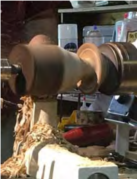
Drill base and then hollow with spindle or roughing gouge to keep from cracking.
