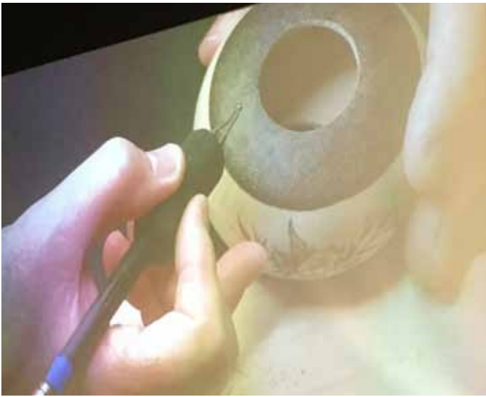
Use a 1/64" ball tip for stippling. Stipple in arbitrary circles. Higher temperature for branding.
