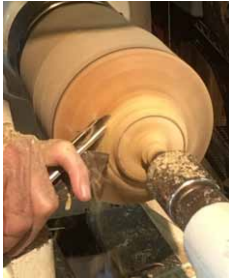
Make tenon. Use side of gouge on end grain to smooth out. Reverse piece on lathe, secure in chuck.
