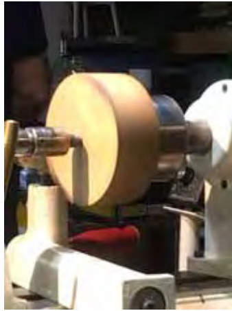
Attach blank with screw, round bowl out with roughing gouge.
