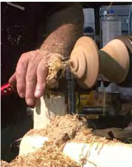
Shear cut top with flute pointing south. Norfolk Pine is full of sand so you'll sharpen tools more often.
