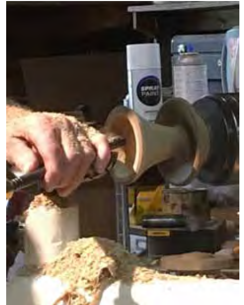
Drill base and then hollow with spindle or roughing gouge to keep from cracking.
