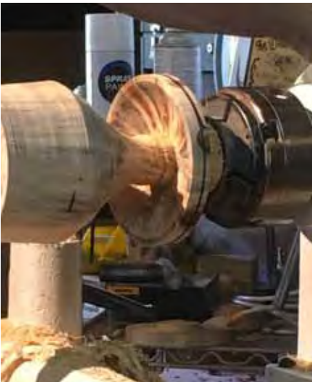
Use parting tool at base of mushroom. Drill and hollow out bottom so it won't crack.
