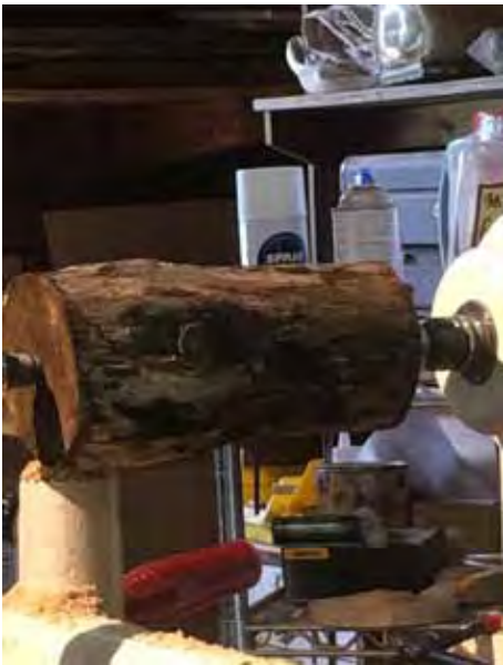
A second mushroom is begun. Smooth out with roughing gouge. Align knots as before.
