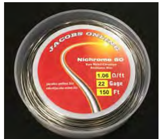
20/22 gauge wire for making nibs.
