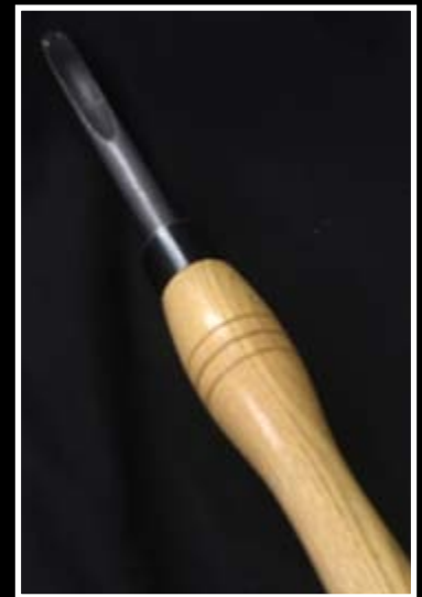
Steve John's Mark Sillay grind for spindle gouge.
