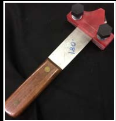
Franck Johannesen designed tool for cutting grooves on back of Russ's sunburst piece.
