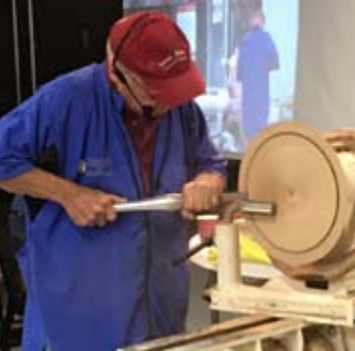
Russ Fellows turns a piece of sycamore to make a wash basin. He cuts from the outside to the inside with a reinforced parting tool. He cuts 5 layers and runs them through a sander. He glues the rings with Tetebond III (waterproof glue) and turns the bowl to a 1/2" thickness.
