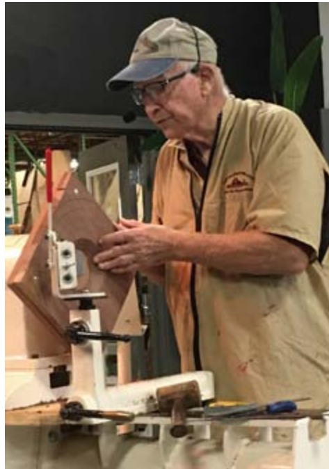
Franck Johannesen uses a One Way Drill Wizard with Chinese high speed steel and Doug Thompson cutters on a Walnut board bolted to a piece of MDF. He cuts each ring at a 45° angle.
