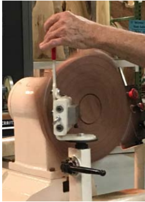
Franck Johannesen uses a One Way Drill Wizard with Chinese high speed steel and Doug Thompson cutters on a Walnut board bolted to a piece of MDF. He cuts each ring at a 45° angle.
