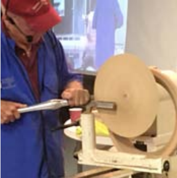
Russ Fellows turns a piece of sycamore to make a wash basin. He cuts from the outside to the inside with a reinforced parting tool. He cuts 5 layers and runs them through a sander. He glues the rings with Tetebond III (waterproof glue) and turns the bowl to a 1/2" thickness.
