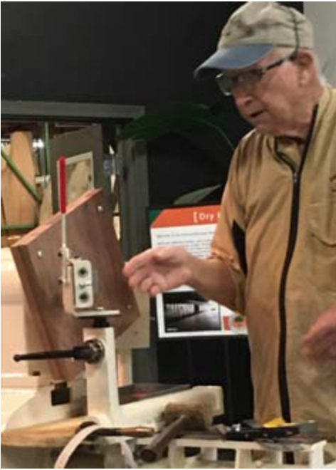
Franck Johannesen uses a One Way Drill Wizard with Chinese high speed steel and Doug Thompson cutters on a Walnut board bolted to a piece of MDF. He cuts each ring at a 45° angle.
