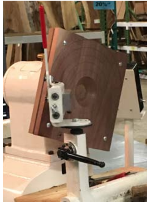
Franck Johannesen uses a One Way Drill Wizard with Chinese high speed steel and Doug Thompson cutters on a Walnut board bolted to a piece of MDF. He cuts each ring at a 45° angle.
