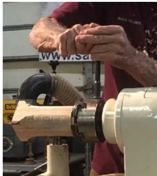
Russ uses Butcher Block Conditioner, a food safe finish. He prepares to turn an on center 3 axis piece.
