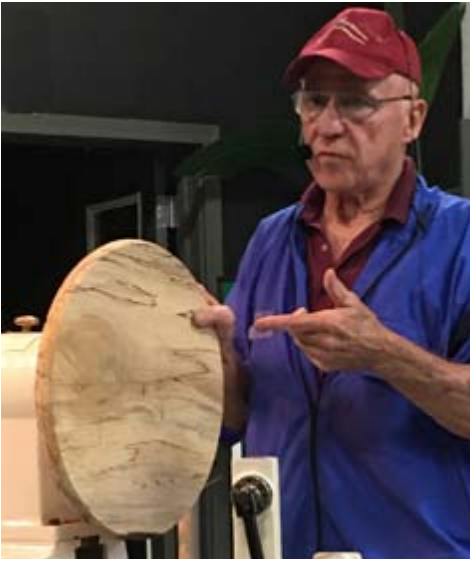
Russ Fellows turns a piece of sycamore to make a wash basin. He cuts from the outside to the inside with a reinforced parting tool. He cuts 5 layers and runs them through a sander. He glues the rings with Tetebond III (waterproof glue) and turns the bowl to a 1/2" thickness.
