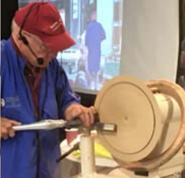
Russ Fellows turns a piece of sycamore to make a wash basin. He cuts from the outside to the inside with a reinforced parting tool. He cuts 5 layers and runs them through a sander. He glues the rings with Tetebond III (waterproof glue) and turns the bowl to a 1/2" thickness.
