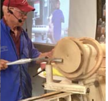
Russ Fellows turns a piece of sycamore to make a wash basin. He cuts from the outside to the inside with a reinforced parting tool. He cuts 5 layers and runs them through a sander. He glues the rings with Tetebond III (waterproof glue) and turns the bowl to a 1/2" thickness.
