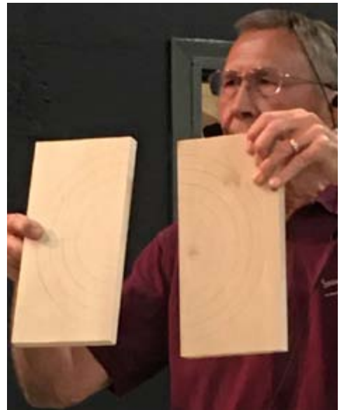
Jim Titze cuts half rings at 45° angle on a band saw and then glues the rings together. He sands flat the smaller diameter of all rings and then glues rings to a block with a tenon in a chuck using the tail stock to center and hold. Then he sands flat the surface of glued rings on lathe.
