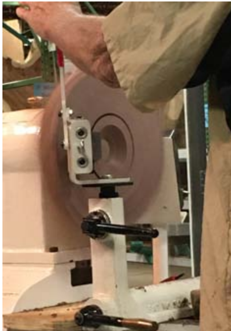
Franck Johannesen uses a One Way Drill Wizard with Chinese high speed steel and Doug Thompson cutters on a Walnut board bolted to a piece of MDF. He cuts each ring at a 45° angle.
