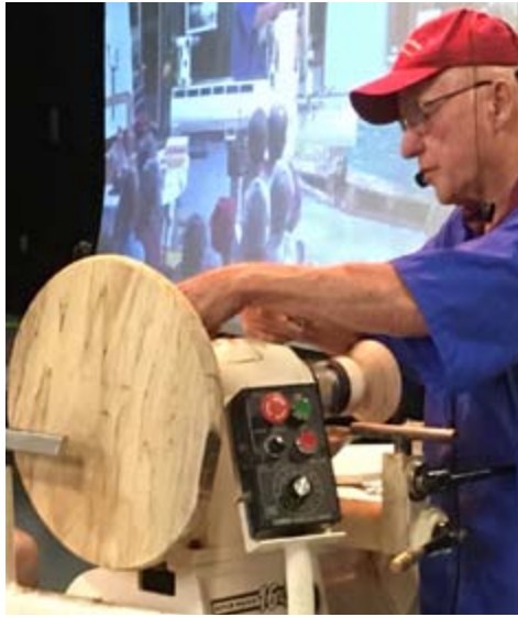
Russ Fellows turns a piece of sycamore to make a wash basin. He cuts from the outside to the inside with a reinforced parting tool. He cuts 5 layers and runs them through a sander. He glues the rings with Tetebond III (waterproof glue) and turns the bowl to a 1/2" thickness.
