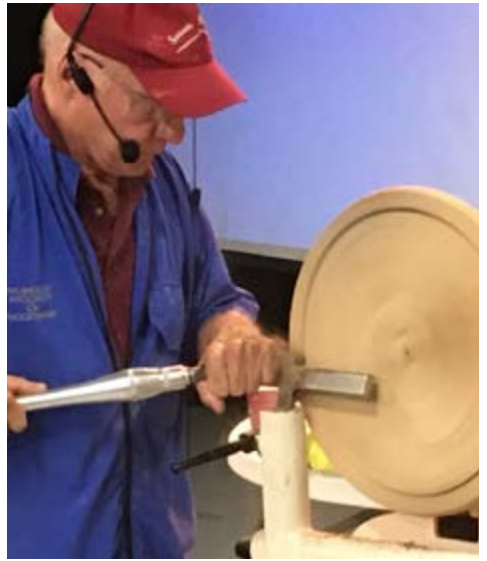
Russ Fellows turns a piece of sycamore to make a wash basin. He cuts from the outside to the inside with a reinforced parting tool. He cuts 5 layers and runs them through a sander. He glues the rings with Tetebond III (waterproof glue) and turns the bowl to a 1/2" thickness.
