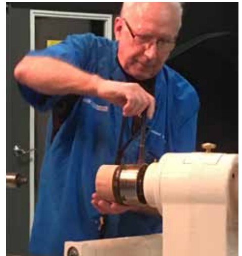
Mount lid to lathe. Shape with spindle gouge and make tenon as small as possible to fit chuck jaws.
