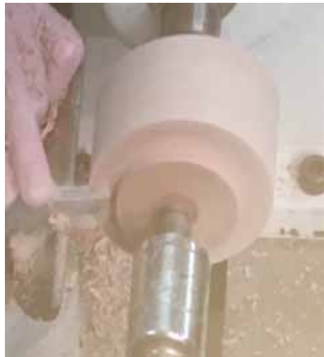
Mount lid to lathe. Shape with spindle gouge and make tenon as small as possible to fit chuck jaws.
