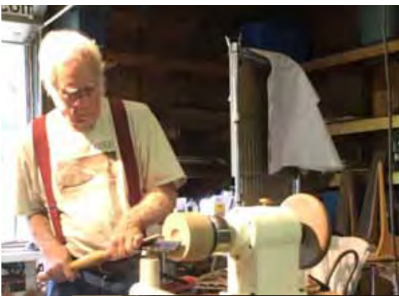
Turn on the bevel of the tool for the best results. The steeper the angle the more shear.
