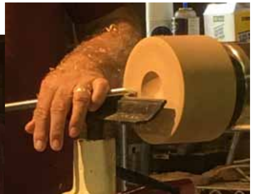
Turn on the bevel of the tool for the best results. The steeper the angle the more shear.
