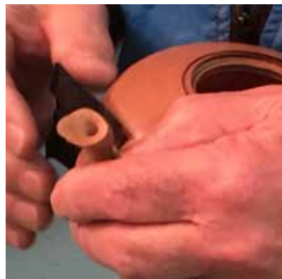
Use carbon paper to help fit spout. Use a micro-grinder to gring off high spots.
