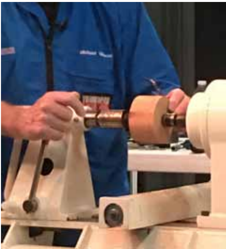
Mount lid to lathe. Shape with spindle gouge and make tenon as small as possible to fit chuck jaws.
