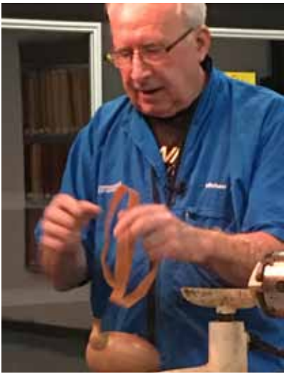
Glue and secure with large rubber or elastic bands.
