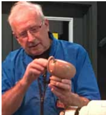
Make 1/4" dowel with with 1/4" wrench. Use steel pins to attach handle. They must be parrallel.
