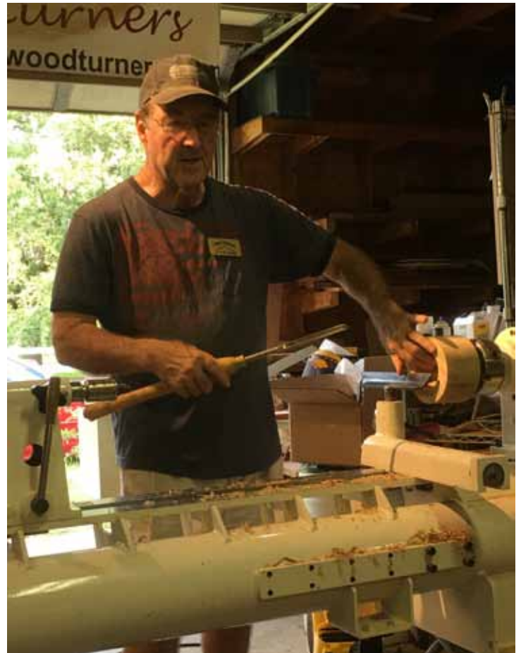
Turn on the bevel of the tool for the best results. The steeper the angle the more shear.
