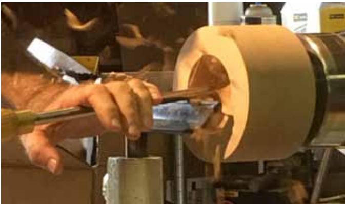
Turn on the bevel of the tool for the best results. The steeper the angle the more shear.
