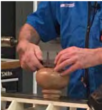
Shear scraper takes care of torn grain. Check size of lid with body of tea pot.
