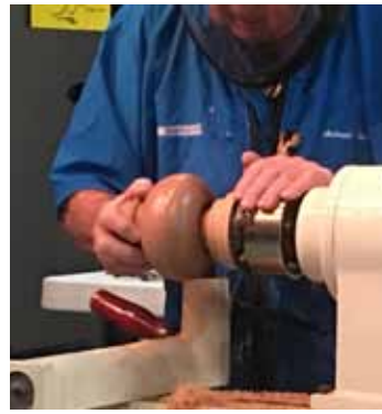
Shear scraper takes care of torn grain. Check size of lid with body of tea pot.
