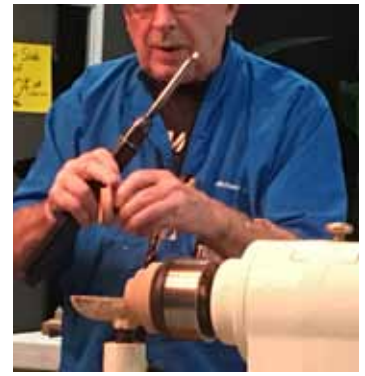
Mount lid to lathe. Shape with spindle gouge and make tenon as small as possible to fit chuck jaws.
