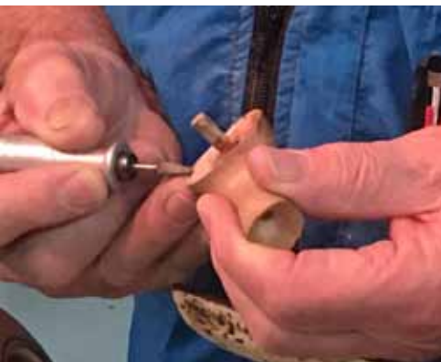
Use carbon paper to help fit spout. Use a micro-grinder to gring off high spots.
