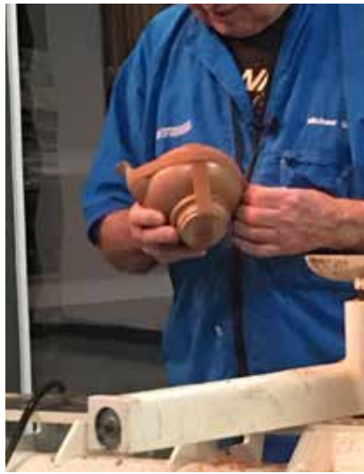
Glue and secure with large rubber or elastic bands.
