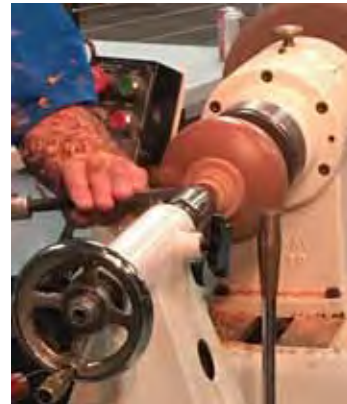
Shear scraper takes care of torn grain. Check size of lid with body of tea pot.
