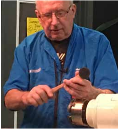
Wooden lid holder for finishing lid. Simple sanding tool.
