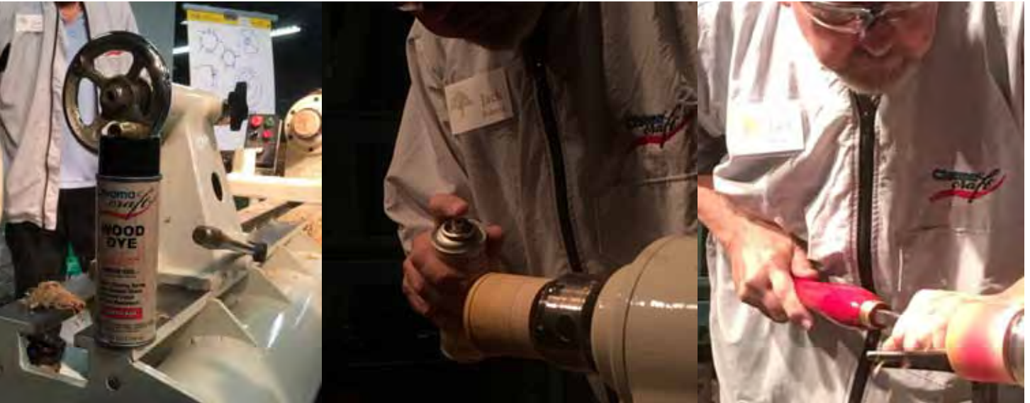
Jack hollows out the bottom. He has done this in the past with Forstner bits, Trent Bosch Hollowing System, Carbide Cutters and/or Easy Wood Tools. The inside is finished with Lacquer Finishing Sealer.
