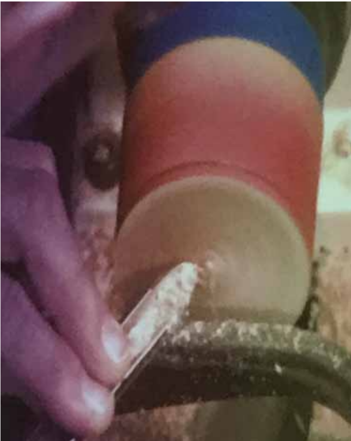
Using a jam chuck Jack finishes turning off the bottom. He uses a pointy tool to detail lines and finishes with sanding sealer and clear lacquer spray on the outside.
