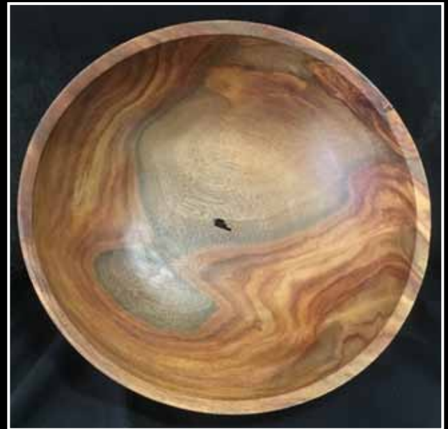
Jim Weeks' Rosewood salad bowl for a wedding gift that developed a hole in the bottom while turning off the tenon.
