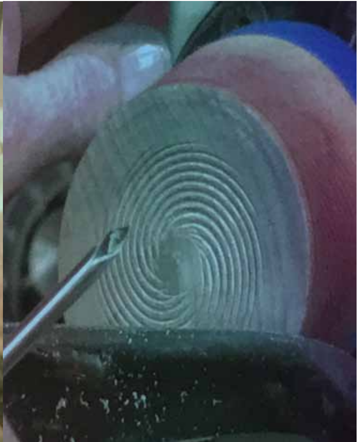
Using a jam chuck Jack finishes turning off the bottom. He uses a pointy tool to detail lines and finishes with sanding sealer and clear lacquer spray on the outside.
