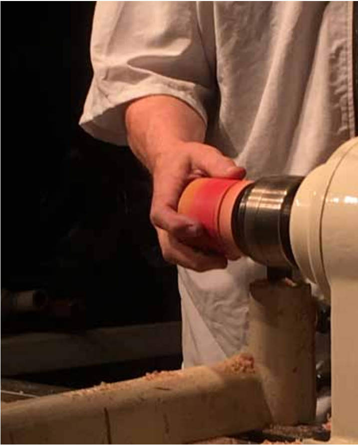
Using a jam chuck Jack finishes turning off the bottom. He uses a pointy tool to detail lines and finishes with sanding sealer and clear lacquer spray on the outside.
