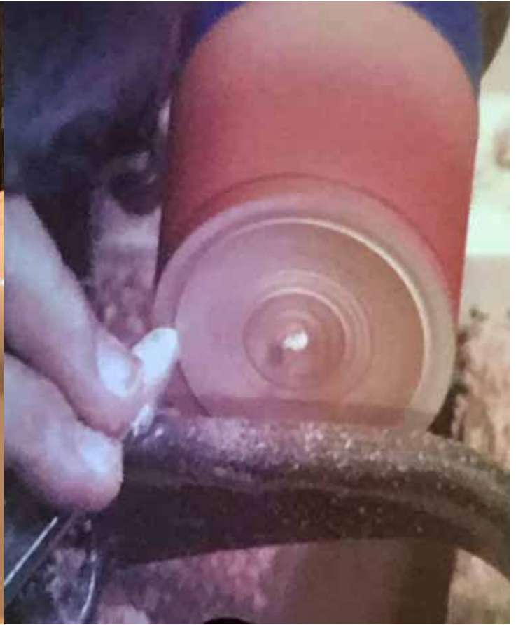
Using a jam chuck Jack finishes turning off the bottom. He uses a pointy tool to detail lines and finishes with sanding sealer and clear lacquer spray on the outside.
