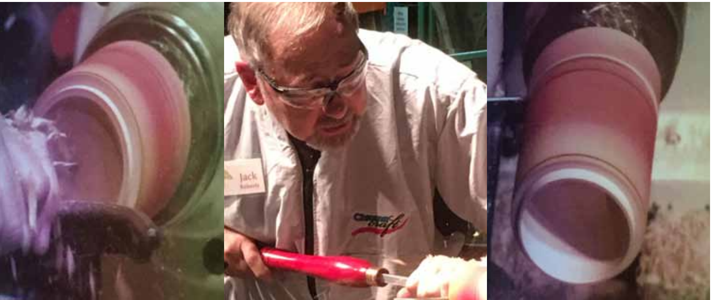
Jack hollows out the bottom. He has done this in the past with Forstner bits, Trent Bosch Hollowing System, Carbide Cutters and/or Easy Wood Tools. The inside is finished with Lacquer Finishing Sealer.
