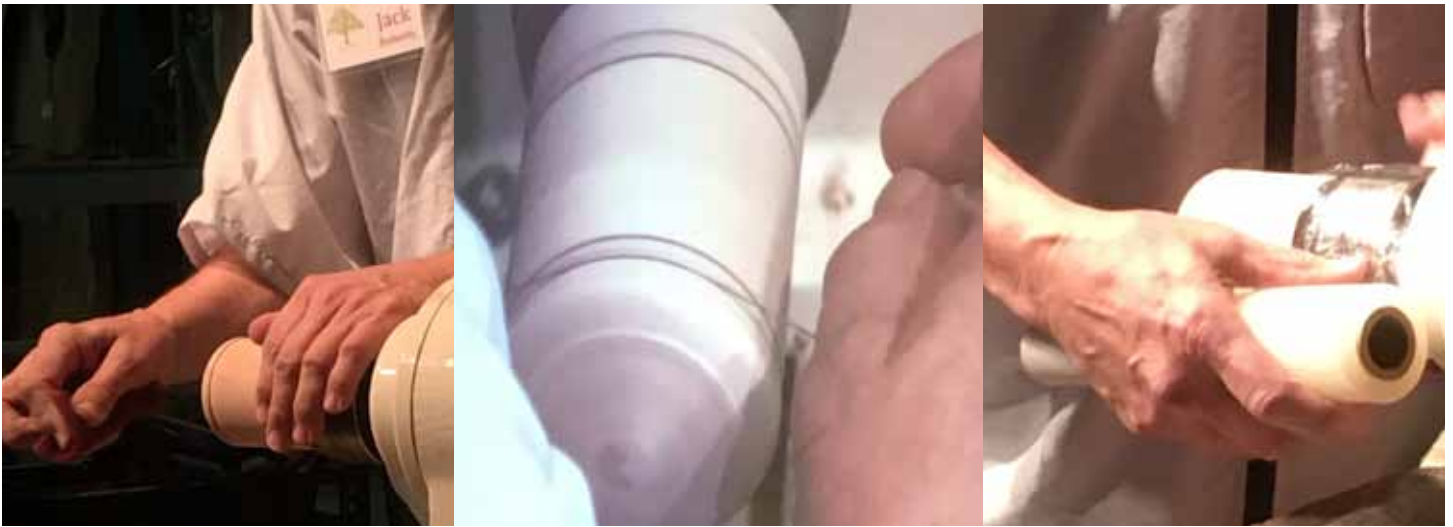
Jack then adds definition to the lines with a wire. He covers his chuck with cling wrap and sprays the sides of box with Chroma craft colored wood dye.
