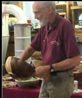
Jim Weeks' Rosewood salad bowl for a wedding gift that developed a hole in the bottom while turning off the tenon.
