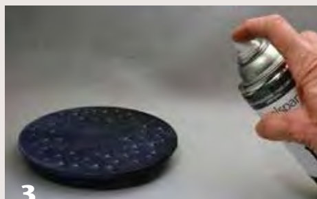
3 Spray a light-colored paint at a shallow angle on one side of the water droplets. Rotate the platter 180 degrees and spray a dark-colored paint on the opposite side.
