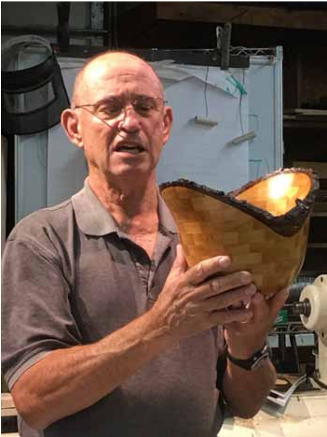
A natural edge, segmented cherry bowl. A chunk from each side is cut off, sanded and then pieces of cherry bark and coffee grounds are added and glued with CA. The bowl is then turned again.
