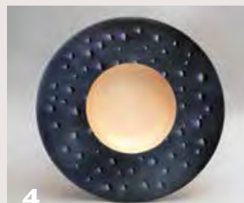
4 After the spray paints have dried and the water has evaporated, finish turning the platter by turning away the center area.
