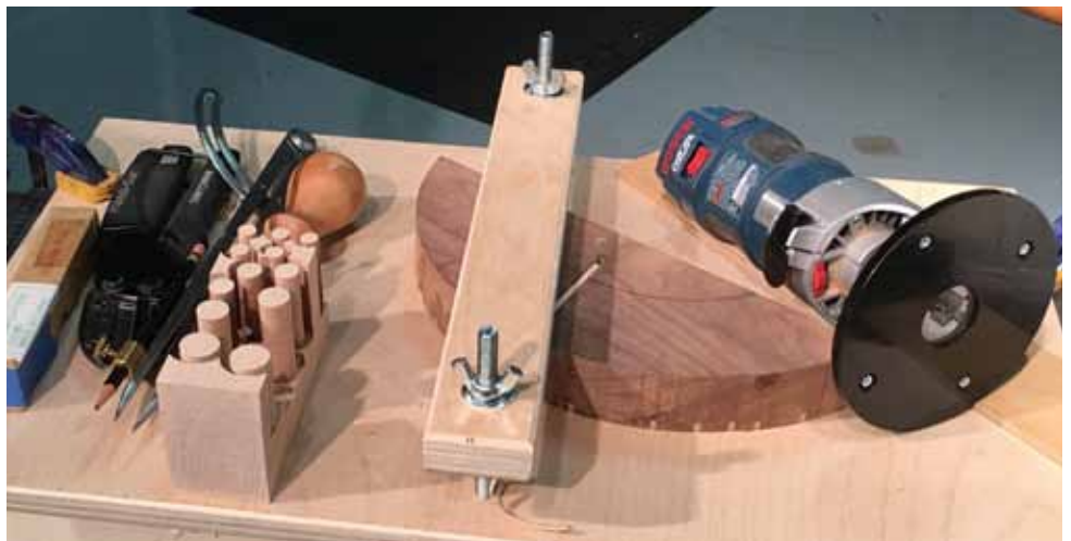
Inlay plugs are in facegrain orientation and sawed into 1/8" wafers.
