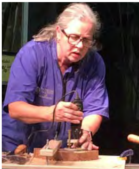
Janet Routes arcs in the blank using a plastic disk template secured with double sided sticky tape.
