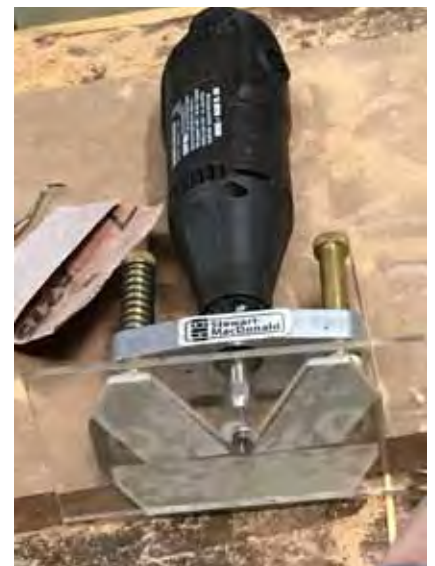
Janet Routes arcs in the blank using a plastic disk template secured with double sided sticky tape.
