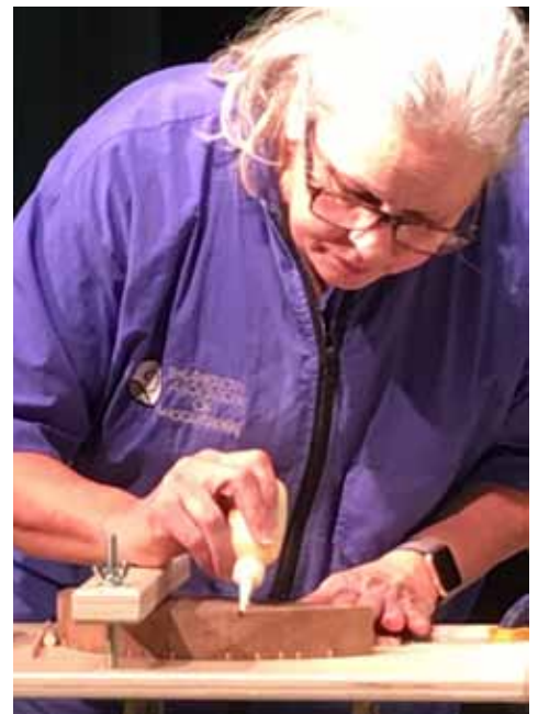
Janet routes, glues and inserts wood strips into the platter blank.
