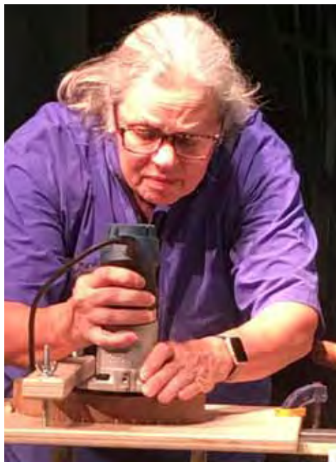
Janet routes, glues and inserts wood strips into the platter blank.
