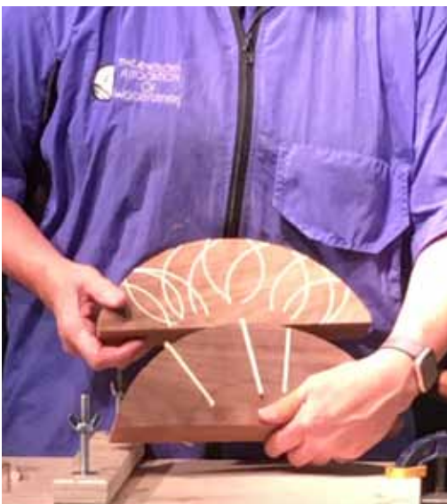
Janet Routes arcs in the blank using a plastic disk template secured with double sided sticky tape.
