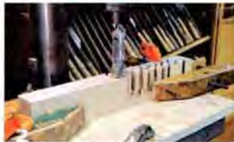
A single board can yield many plugs of varying diameters, and each plug may yield two or more pieces for inlay.
