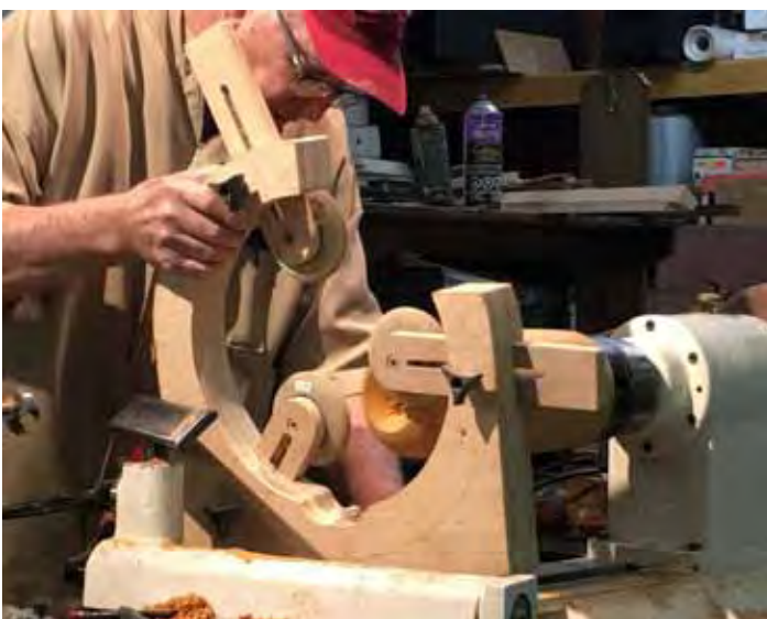
Hollowing with 3/8" high speed cutting tool edge and reverse lathe speed direction.
