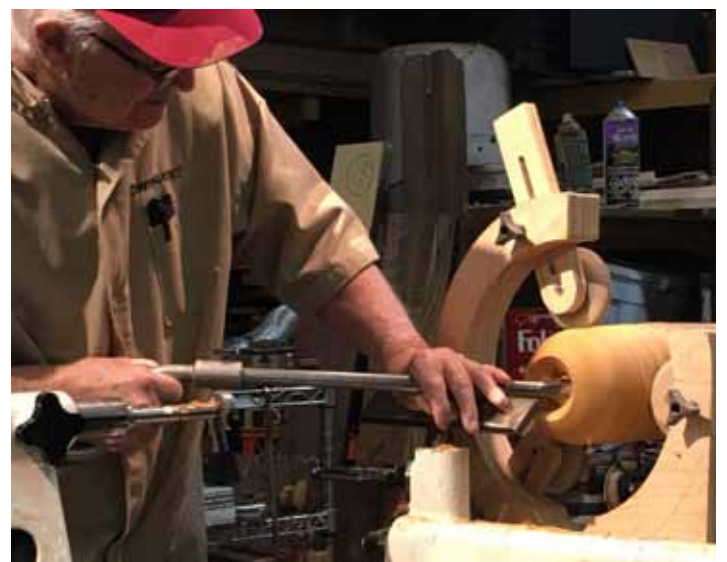
Hollowing with 3/8" high speed cutting tool edge and reverse lathe speed direction.
