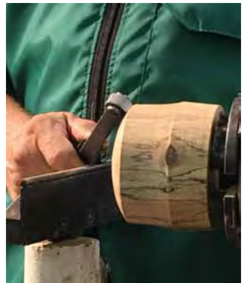
Texturing end grain on box top and using the Wagner embossing tool.
