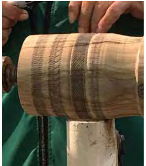
Turning the tool at various angles produces different patterns.
