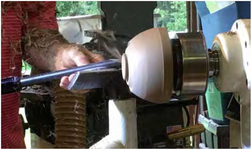
Steve marks face for tenon with pen. He uses a spindle gouge to make an undercut on the tenon, and cleans up/flattens face.
