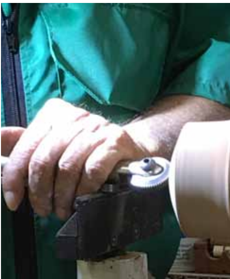
Texturing end grain on box top and using the Wagner embossing tool.
