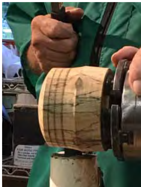
Texturing end grain on box top and using the Wagner embossing tool.
