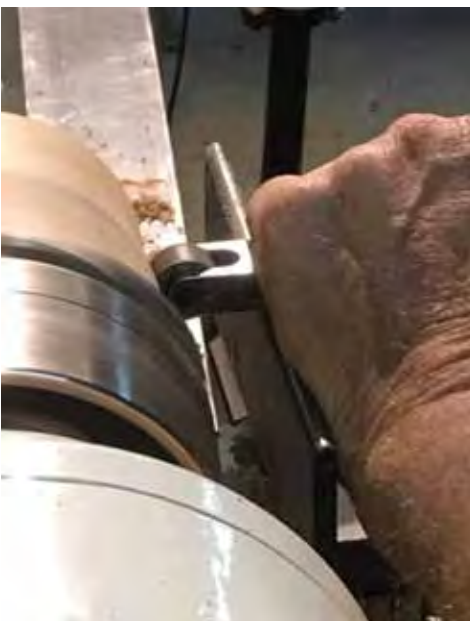
Texturing end grain on box top and using the Wagner embossing tool.
