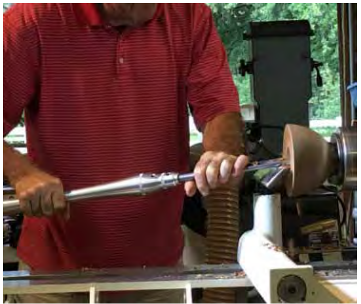
Starting from the far right he swings the handle towards his body.
