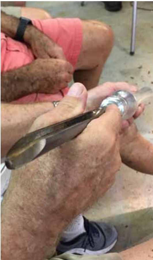
Steve uses a 55 - 60° bevel on his gouges. He finishes his bowls with EEE-Ultra Shine.
