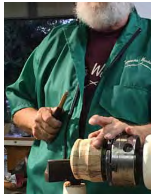
Texturing end grain on box top and using the Wagner embossing tool.
