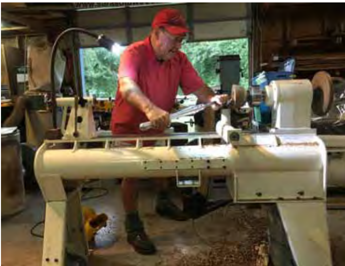
Starting from the far right he swings the handle towards his body.
