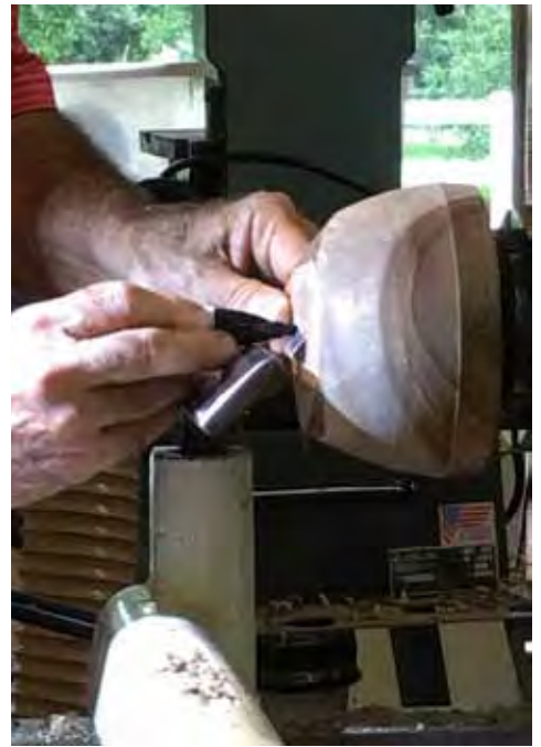
Steve marks face for tenon with pen. He uses a spindle gouge to make an undercut on the tenon, and cleans up/flattens face.
