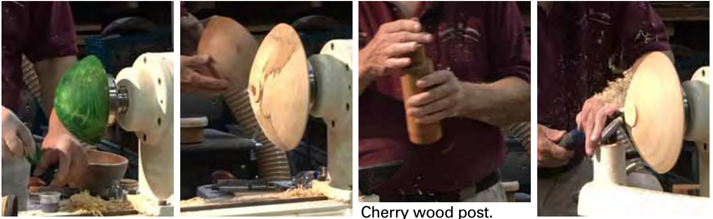
Franck mounts the wig stand top in a chuck and cleans it up. He then sands it thru 320 grit and applies Transol Powdered Solvent Dye made with 2-3 drops of dye added to Denatured Alcohol.
