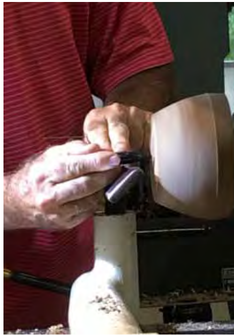
Steve marks face for tenon with pen. He uses a spindle gouge to make an undercut on the tenon, and cleans up/flattens face.
