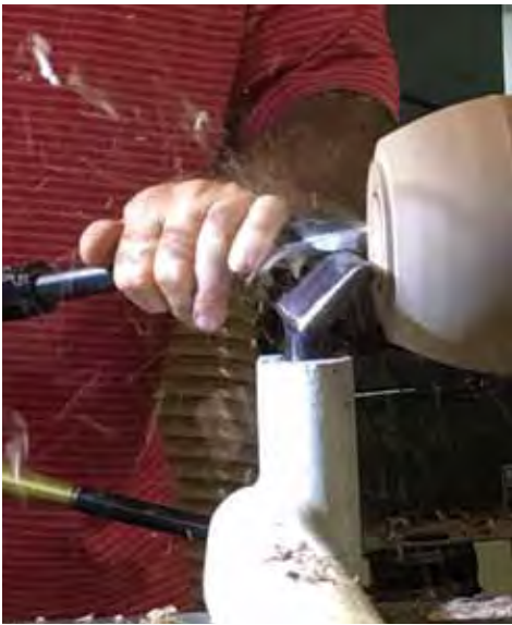
Steve marks face for tenon with pen. He uses a spindle gouge to make an undercut on the tenon, and cleans up/flattens face.
