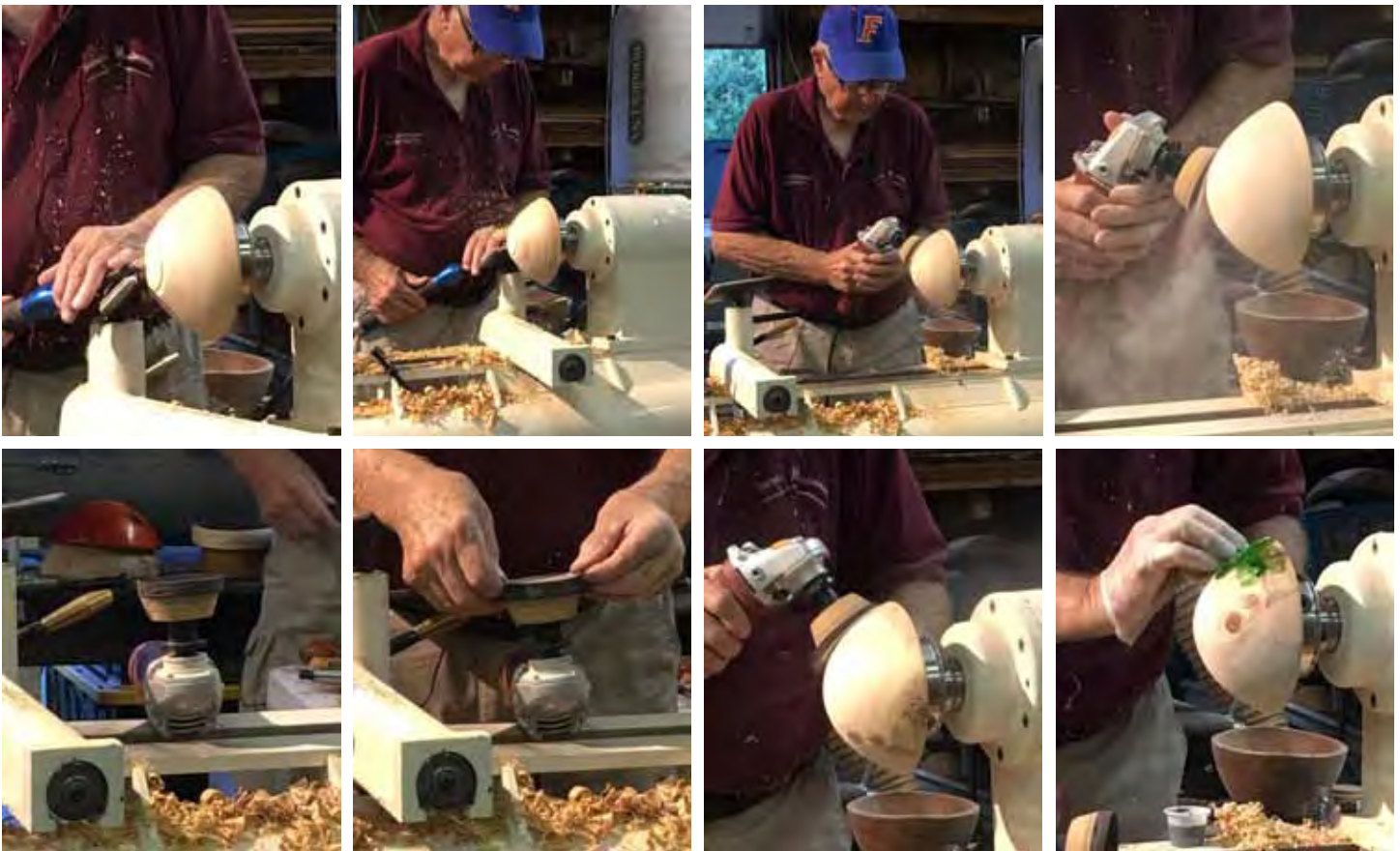
Franck mounts the wig stand top in a chuck and cleans it up. He then sands it thru 320 grit and applies Transol Powdered Solvent Dye made with 2-3 drops of dye added to Denatured Alcohol.
