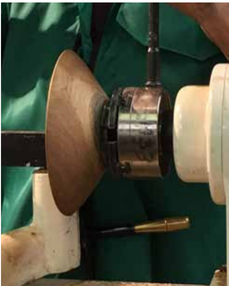
Turning the tool at various angles produces different patterns.
