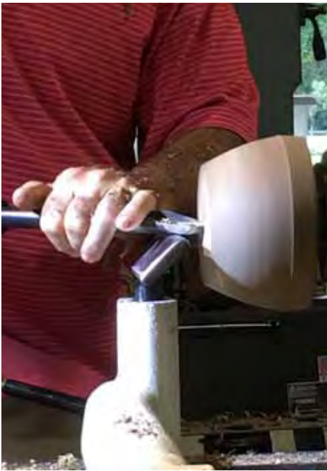
Steve marks face for tenon with pen. He uses a spindle gouge to make an undercut on the tenon, and cleans up/flattens face.
