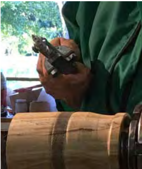
Turning the tool at various angles produces different patterns.
