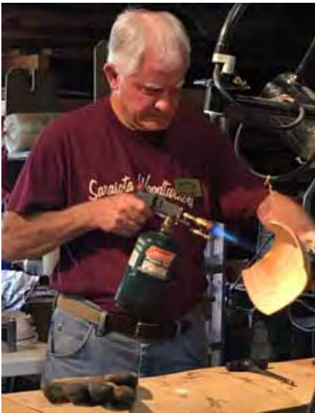
Torch burning China Berry and then sanding with 600 grit paper brings out the grain and takes away the burn.
