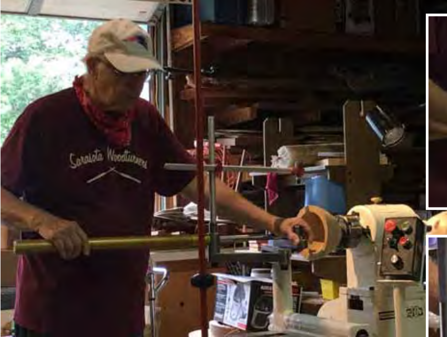
Franck Johannesen demonstrating the Trent Bosch Hollowing System which he now sells.
