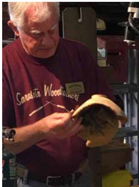
Torch burning China Berry and then sanding with 600 grit paper brings out the grain and takes away the burn.
