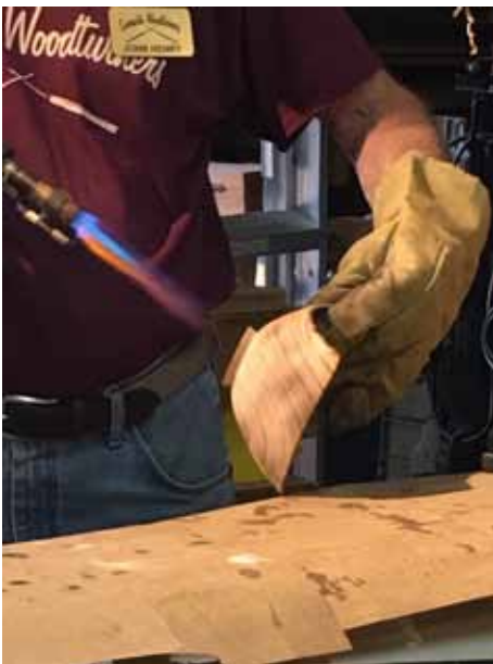
Torch burning China Berry and then sanding with 600 grit paper brings out the grain and takes away the burn.
