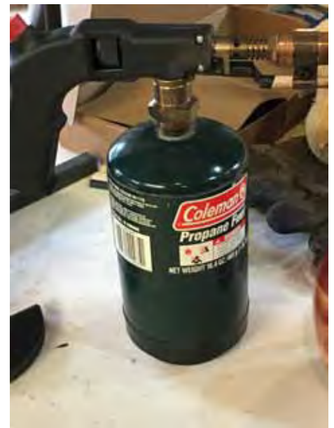
Torch burning China Berry and then sanding with 600 grit paper brings out the grain and takes away the burn.
