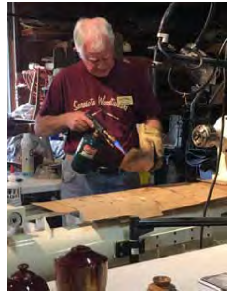
Torch burning China Berry and then sanding with 600 grit paper brings out the grain and takes away the burn.
