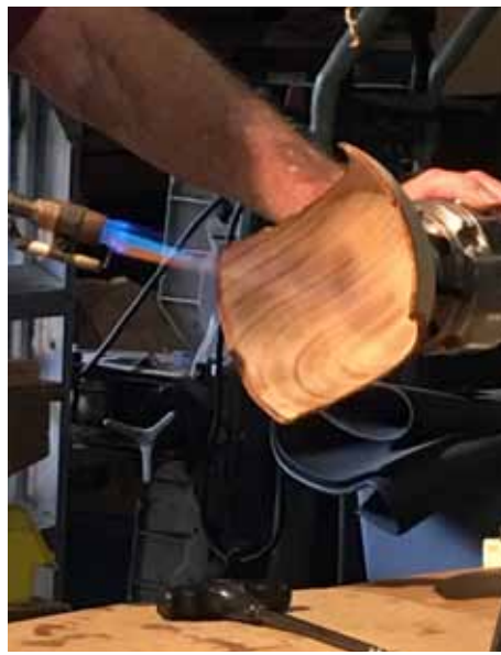
Torch burning China Berry and then sanding with 600 grit paper brings out the grain and takes away the burn.
