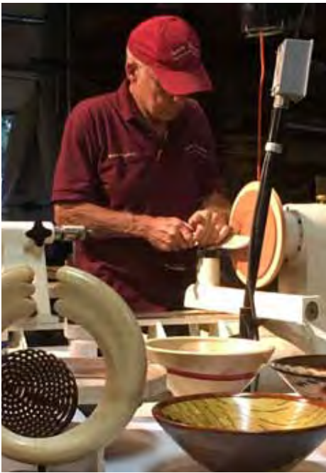
Rings can be cut out on the lathe or cut at a 45 degree angle on a bandsaw.
