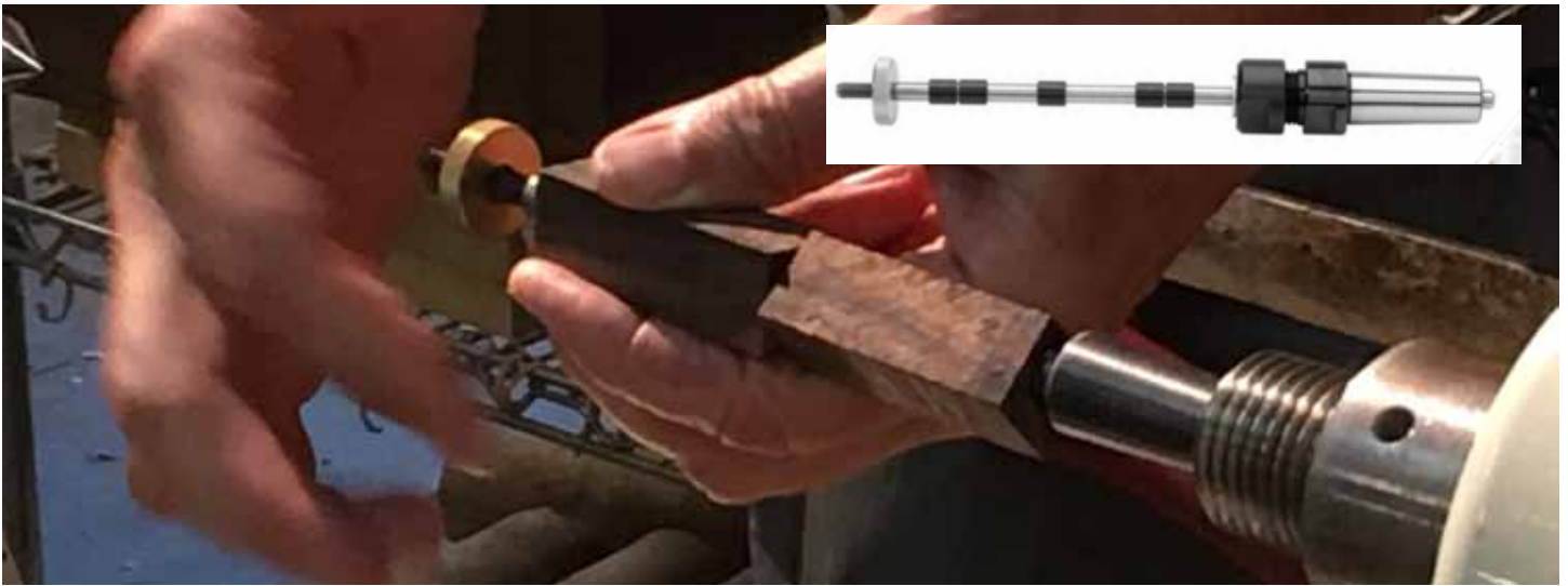
2 MT Penn Mandrel. Insert is a 2 MT Maxi-Mandrel.
