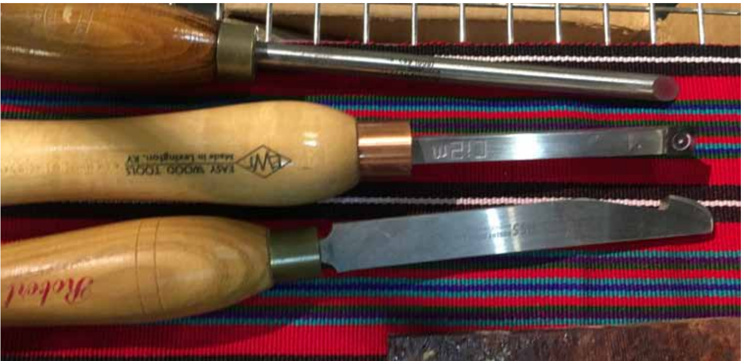
Jim's Henry Taylor Coving Tool, Easy Wood R2 Rougher and Robert Sorby Negative Rake Scraper .
