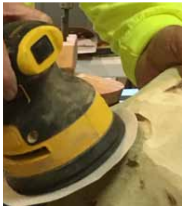
Using a 60-80 grit disk sander, he smooths the transitions between high and low. A 6" paper on a 5" sanders hits the hills and valleys.
