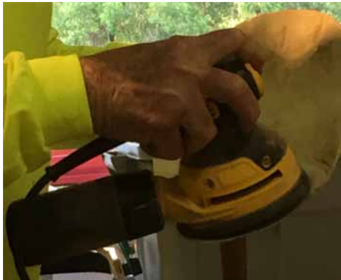
Using a 60-80 grit disk sander, he smooths the transitions between high and low. A 6" paper on a 5" sanders hits the hills and valleys.
