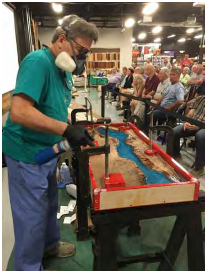
Norm stirs the epoxy resin and then uses a benzomatic torch to remove the remaining bubbles.
