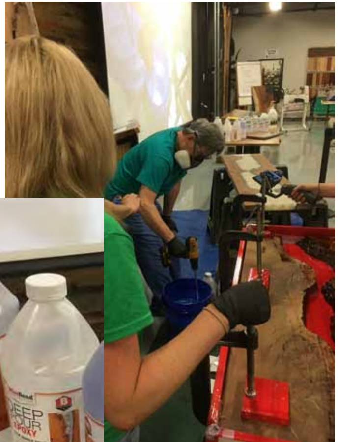
Dave Jadin of Advantage Lumber narrates the epoxy river table demonstration. Norm and Tony Moore prepare the Epe Burl slabs. They level the table then secure the wood with bar clamps to prevent the wood from floating in the epoxy.
