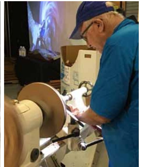
12 segmented rings glued to a MDF board. Franck cutting rings on the lathe.
