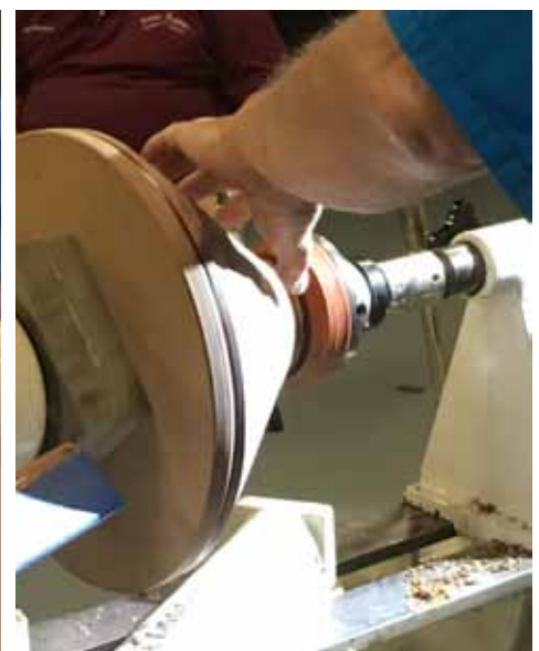
Using a 7/8" roughing gouge Franck makes light cuts to the outside of the bowl.
