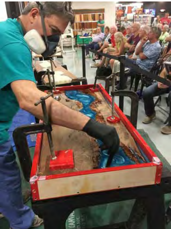
Norm stirs the epoxy resin and then uses a benzomatic torch to remove the remaining bubbles.
