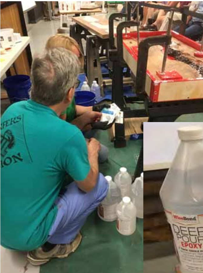
Dave Jadin of Advantage Lumber narrates the epoxy river table demonstration. Norm and Tony Moore prepare the Epe Burl slabs. They level the table then secure the wood with bar clamps to prevent the wood from floating in the epoxy.
