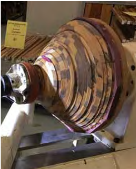
12 segmented rings glued to a MDF board. Franck cutting rings on the lathe.
