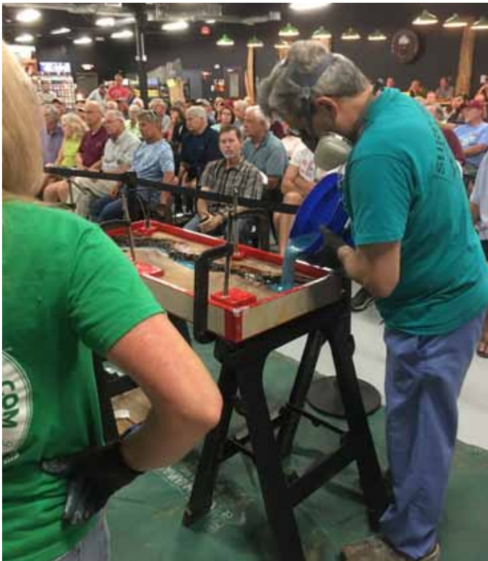
Slowly pouring the epoxy resin into the “river” of the Epe Burl slabs.
