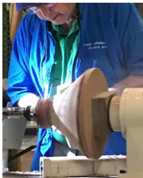
Using a 7/8" roughing gouge Franck makes light cuts to the outside of the bowl.
