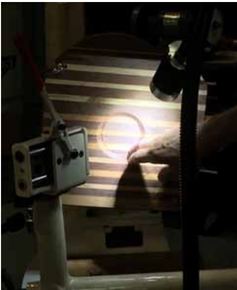
12 segmented rings glued to a MDF board. Franck cutting rings on the lathe.
