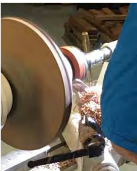
Using a 7/8" roughing gouge Franck makes light cuts to the outside of the bowl.
