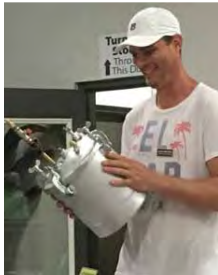
Pressure pot makes bubbles smaller, 40-45 psi. Favorite tools for turning epoxy - EasyWood Carbide tools, Doug Thompson Bowl Gouge, Negative Rage Scraper.
