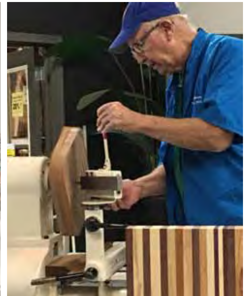
12 segmented rings glued to a MDF board. Franck cutting rings on the lathe.
