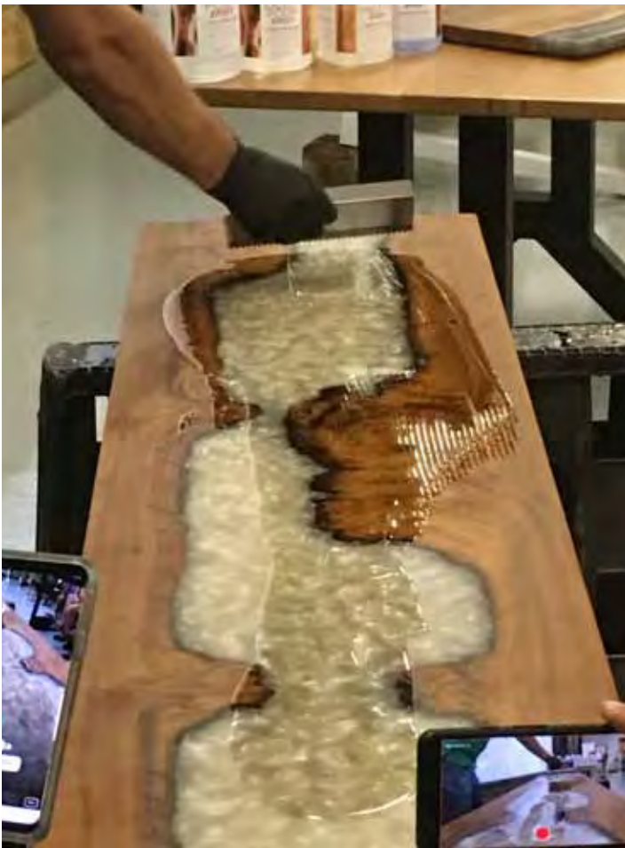
Dave coats and spreads the epoxy on the table top.
