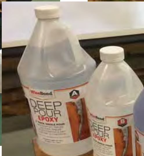
Mixing and stirring the Deep Pour Epoxy A and B at a 2 to 1 ratio.
