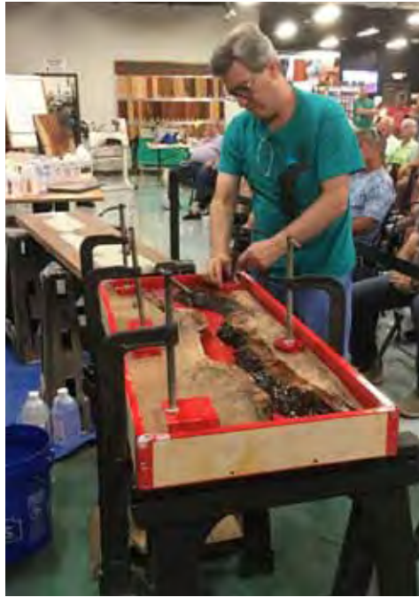
Dave Jadin of Advantage Lumber narrates the epoxy river table demonstration. Norm and Tony Moore prepare the Epe Burl slabs. They level the table then secure the wood with bar clamps to prevent the wood from floating in the epoxy.
