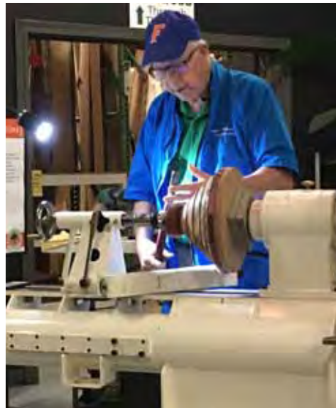
12 segmented rings glued to a MDF board. Franck cutting rings on the lathe.
