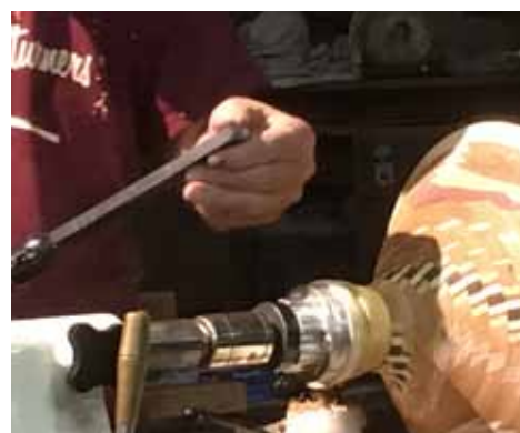
Grain direction changes. Use bowl 50° gouge maintaining firm pressure on tool rest.
