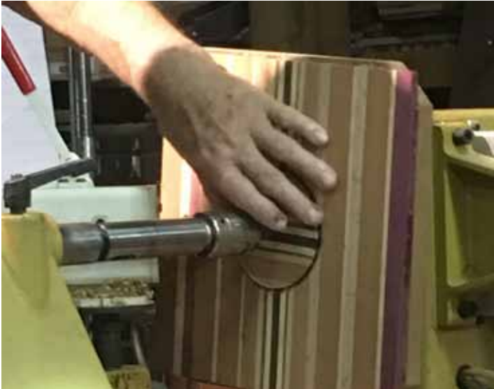
Franck Johannesen's "modified" Oneway Drill Wizard with a mounted parting tool blade.
