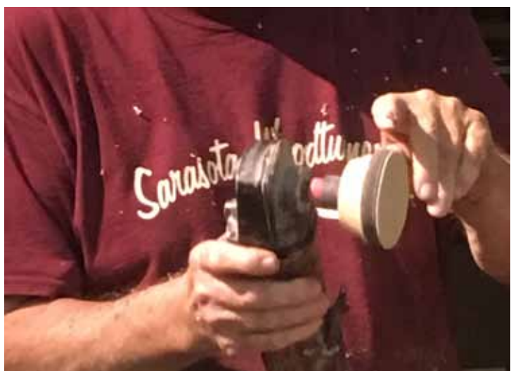
Using angle grinder with pad, sand with 80 grit and go to 400-600 grit. Keep cool, don't soften glue.
