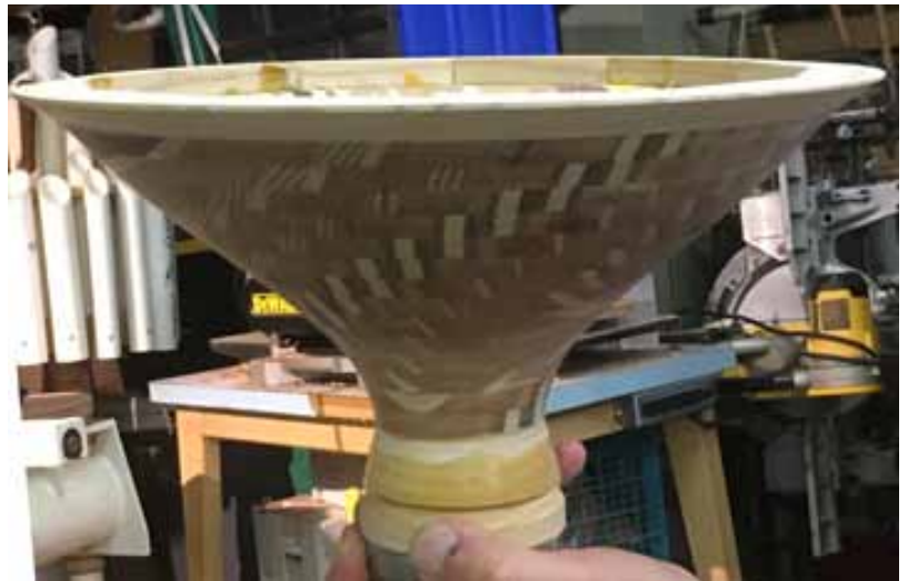
Seal outside of bowl with coat of 3408, let dry and carefully cut bowl off backer board.
