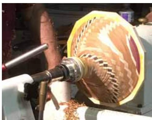
Franck finishes turning with Thompson Heavy Duty Scraper.
