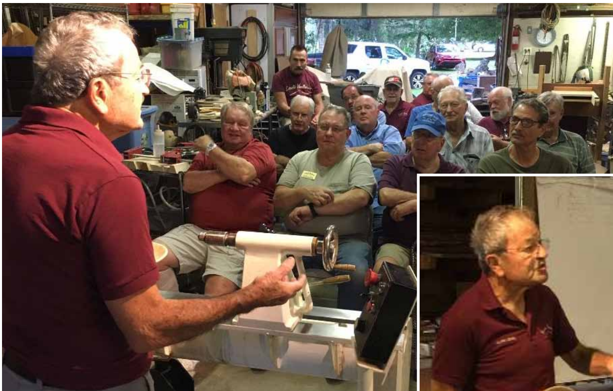
Alan Levin demonstrates his method for centering a bowl on a vacuum chuck.
