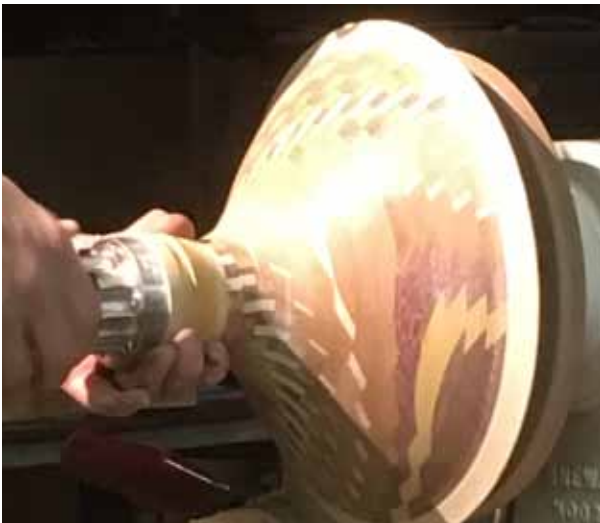
Seal outside of bowl with coat of 3408, let dry and carefully cut bowl off backer board.
