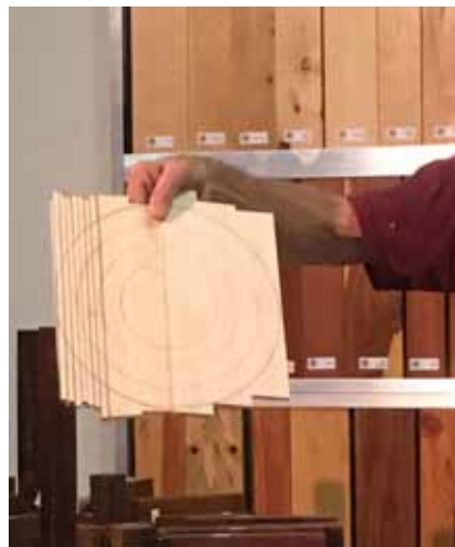
Glue with Titebond III, hold between MDF boards with tail stock and then secure with speed clamps.
