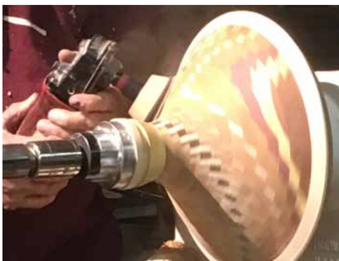
Using angle grinder with pad, sand with 80 grit and go to 400-600 grit. Keep cool, don't soften glue.
