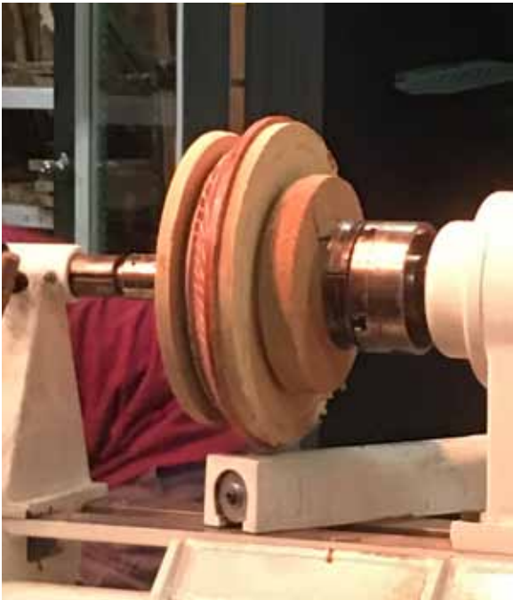
Glue with Titebond III, hold between MDF boards with tail stock and then secure with speed clamps.
