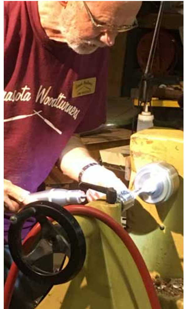
Drilling (1/2" Forstner bit), then hollowing (Simon Hope 6mm cutter and Sorby Minature) to approximately 1/8" thick and then parting the ornament.
