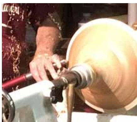
Franck finishes turning with Thompson Heavy Duty Scraper.
