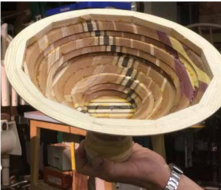
Remount bowl on lathe and slowly trim the inside. It will become quite thin. Start from the rim.
