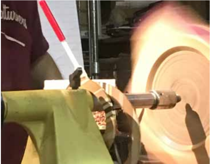
Franck Johannesen's "modified" Oneway Drill Wizard with a mounted parting tool blade.
