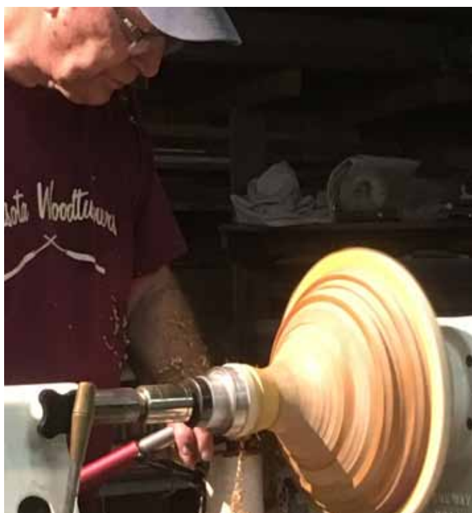
Grain direction changes. Use bowl 50° gouge maintaining firm pressure on tool rest.
