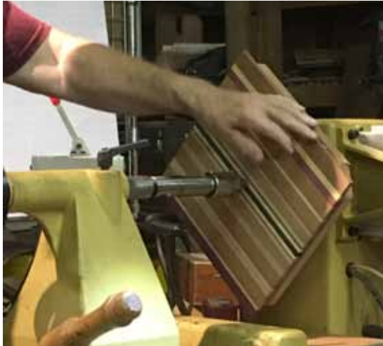
Franck Johannesen's "modified" Oneway Drill Wizard with a mounted parting tool blade.
