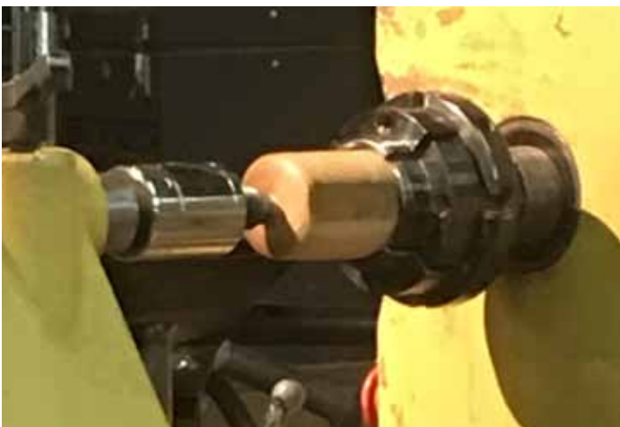
Drilling, then hollowing the ornament.
