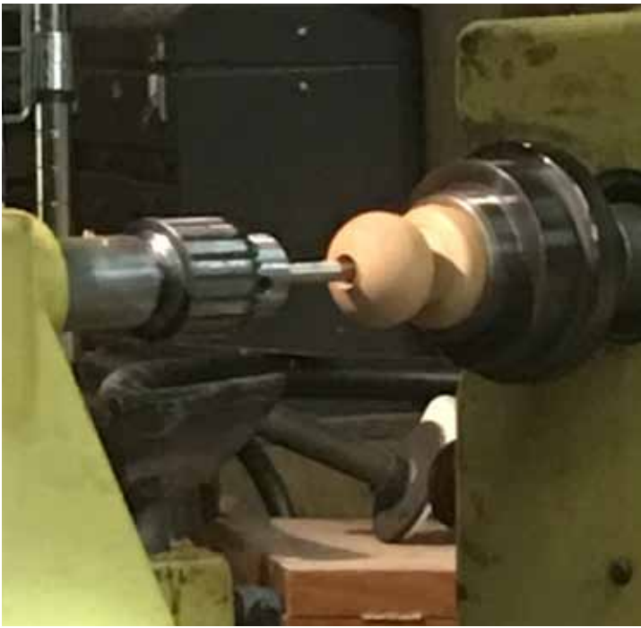
Drilling (1/2" Forstner bit), then hollowing (Simon Hope 6mm cutter and Sorby Minature) to approximately 1/8" thick and then parting the ornament.
