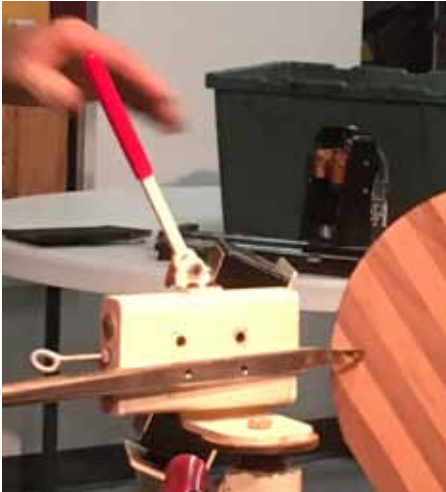
Franck Johannesen's "modified" Oneway Drill Wizard with a mounted parting tool blade.
