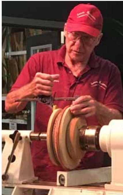
Glue with Titebond III, hold between MDF boards with tail stock and then secure with speed clamps.
