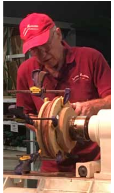
Glue with Titebond III, hold between MDF boards with tail stock and then secure with speed clamps.
