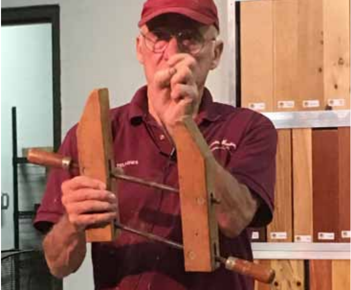
Gently hold rings together with clamp.
