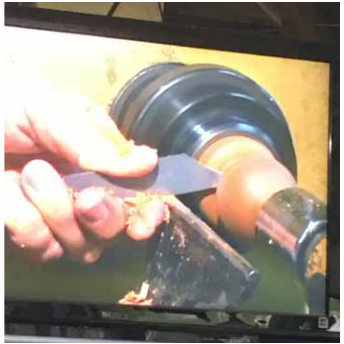
Drilling (1/2" Forstner bit), then hollowing (Simon Hope 6mm cutter and Sorby Minature) to approximately 1/8" thick and then parting the ornament.
