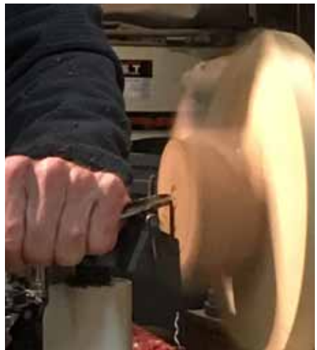
Mount and then hollow with a small gouge. Then cut in half with band saw.
