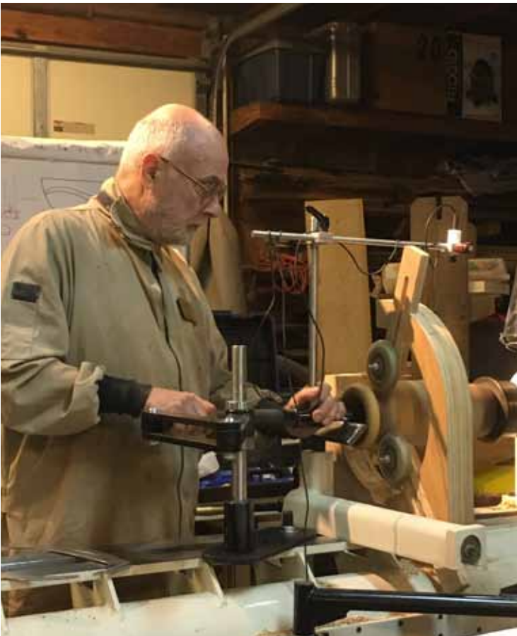
Steady Rest, made of cabinet quality plywood by Tom Falcone , eliminates much of the vibration.
