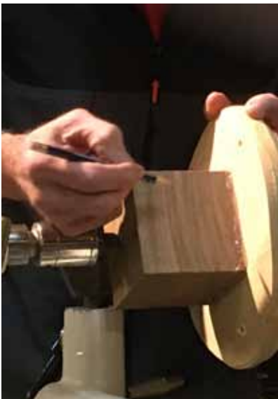
Russ draws the round shape on the block and uses a hemisphere template to check size and shape.
