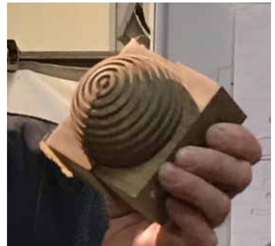
Mount and then hollow with a small gouge. Then cut in half with band saw.
