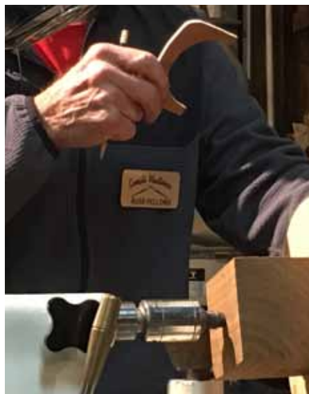
Russ draws the round shape on the block and uses a hemisphere template to check size and shape.
