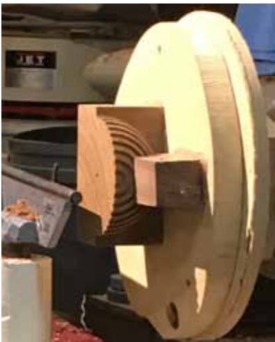
Mount and then hollow with a small gouge. Then cut in half with band saw.
