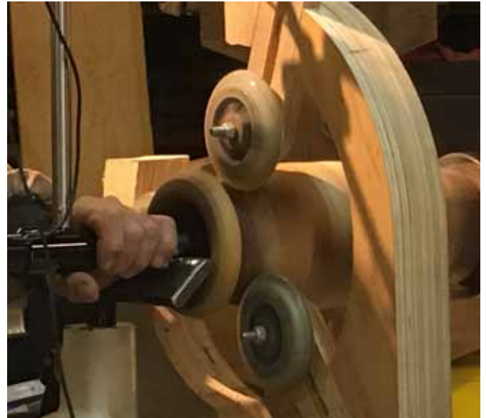
Steady Rest, made of cabinet quality plywood by Tom Falcone , eliminates much of the vibration.
