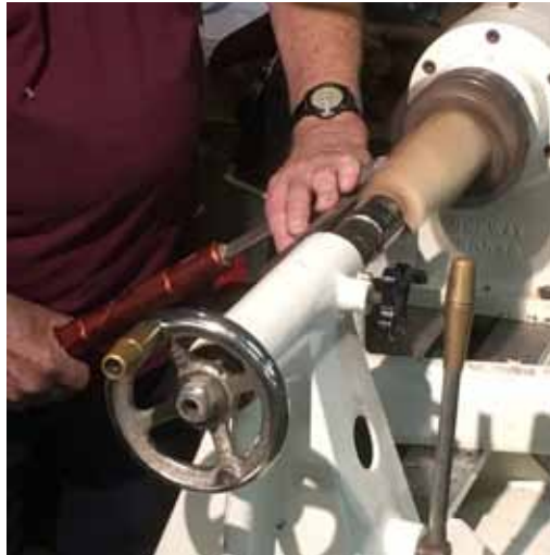
Thompson Large Skew, raise handle till it starts to cut, then hold and move. Control with thumb.
