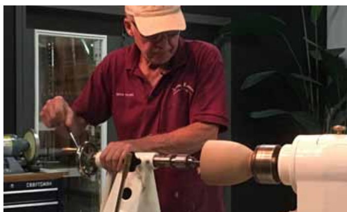
Drilling before hollowing.
