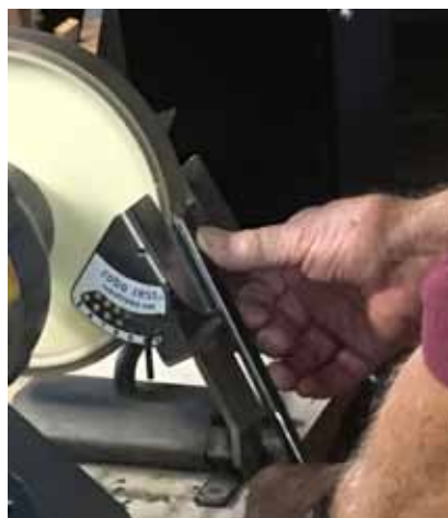
Sharpened at 30° and honed to remove burr.
