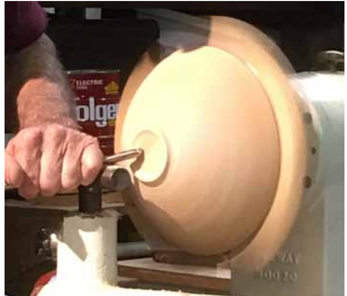
Shape outside first using small bowl gouge. Remove outer part of the tenon.
