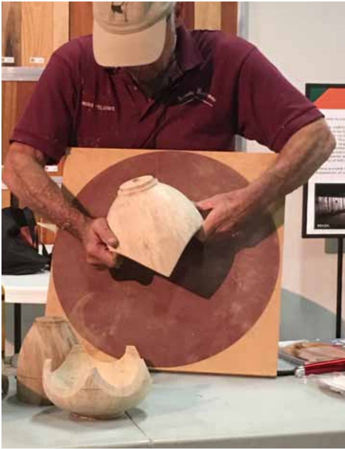
Make three cuts on 45 degree angled band saw 4, then lightly sand edges gently on sanding board.
