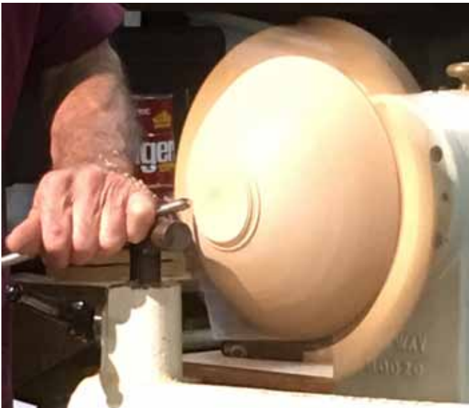
Shape outside first using small bowl gouge. Remove outer part of the tenon.
