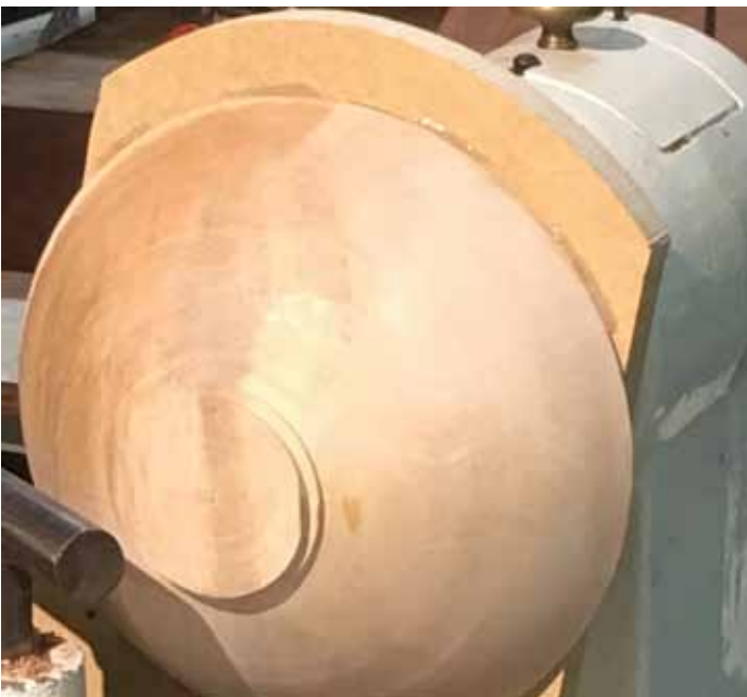
Bowl is hot glued to backing board.
