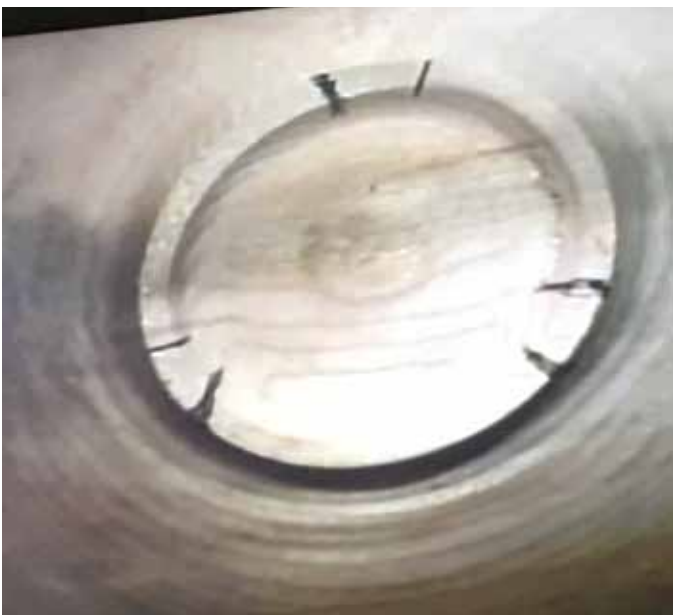
Place bowl on flat surface and grind with a Dremel tool or a Proxxon Longneck Angle Grinder.
