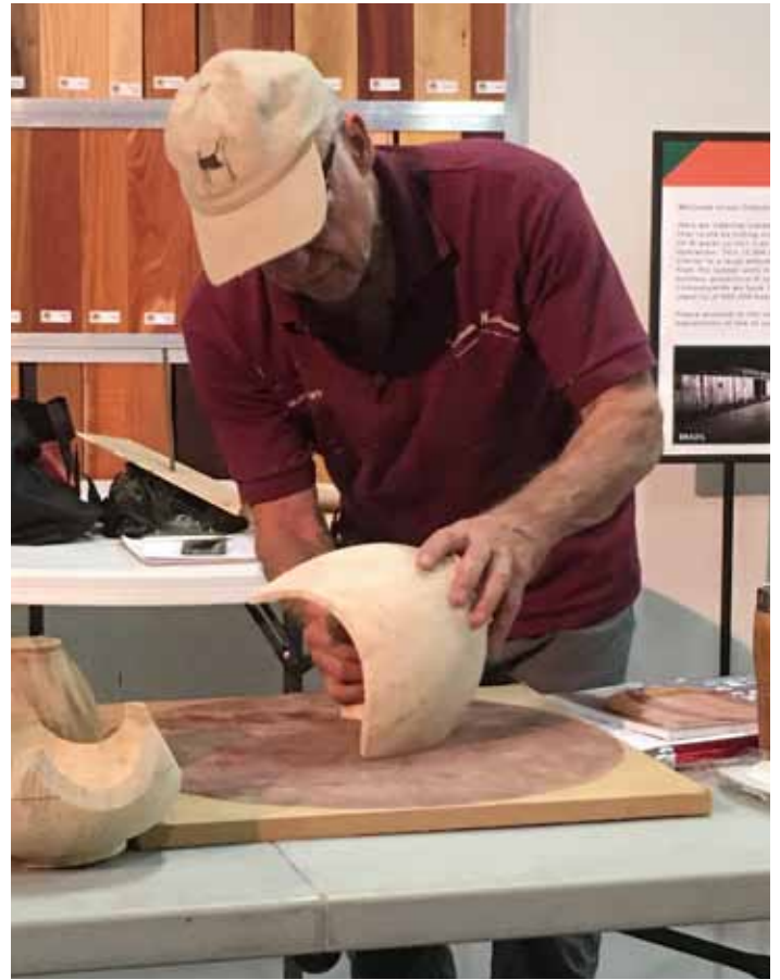
Make three cuts on 45 degree angled band saw 4, then lightly sand edges gently on sanding board.
