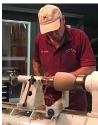
Turning a wing bowl is difficult to turn as grain goes in all directions and wings break off easily.
