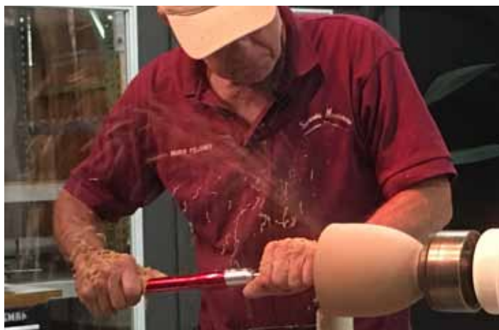
Hollowing with a Harrison Carbide Tip Wood Lathe Tool.
