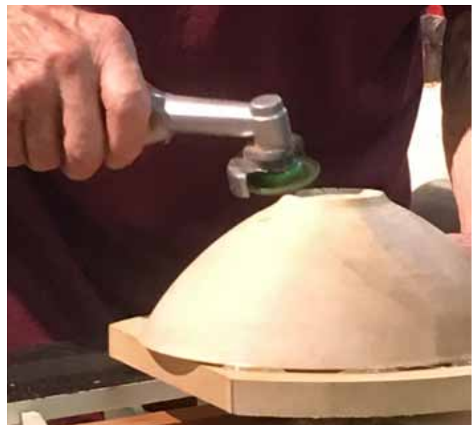
Place bowl on flat surface and grind with a Dremel tool or a Proxxon Longneck Angle Grinder.
