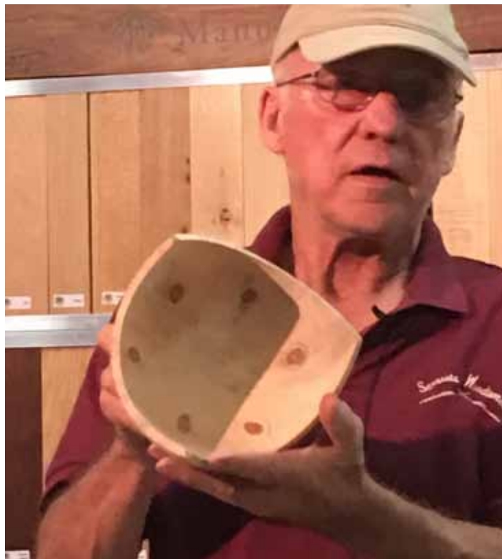
Turning a wing bowl is difficult to turn as grain goes in all directions and wings break off easily.
