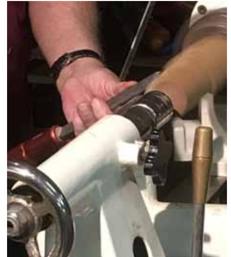
Thompson Large Skew, raise handle till it starts to cut, then hold and move. Control with thumb.
