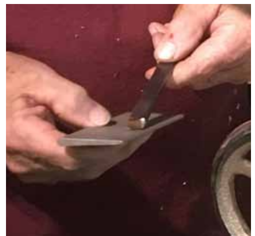
Sharpened at 30° and honed to remove burr.
