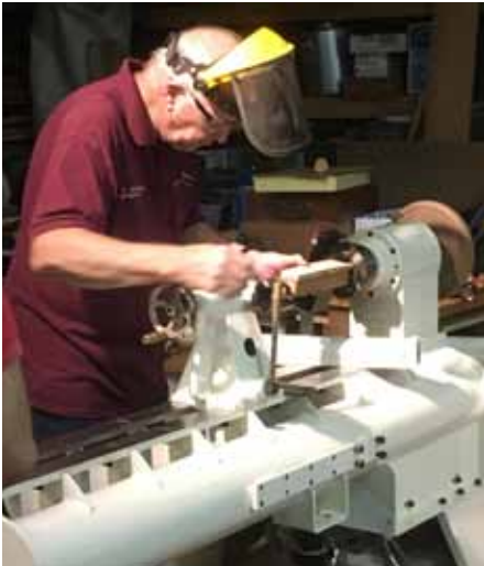
Attach wood with Standard Oneway Spring Loaded Safedrive.
