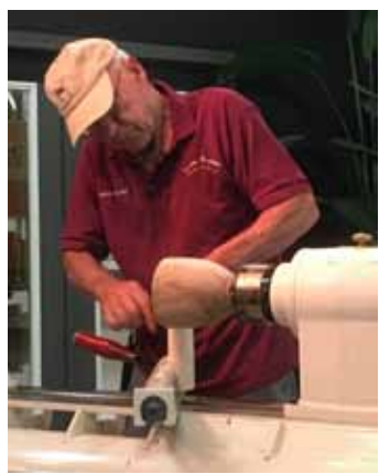
Turning a wing bowl is difficult to turn as grain goes in all directions and wings break off easily.
