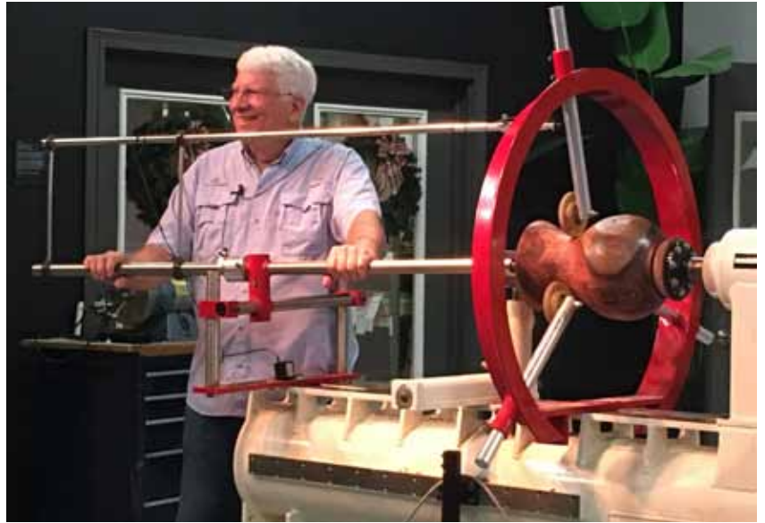
Clark Deep Hollowing System with Companion Clark Steady Rest.
