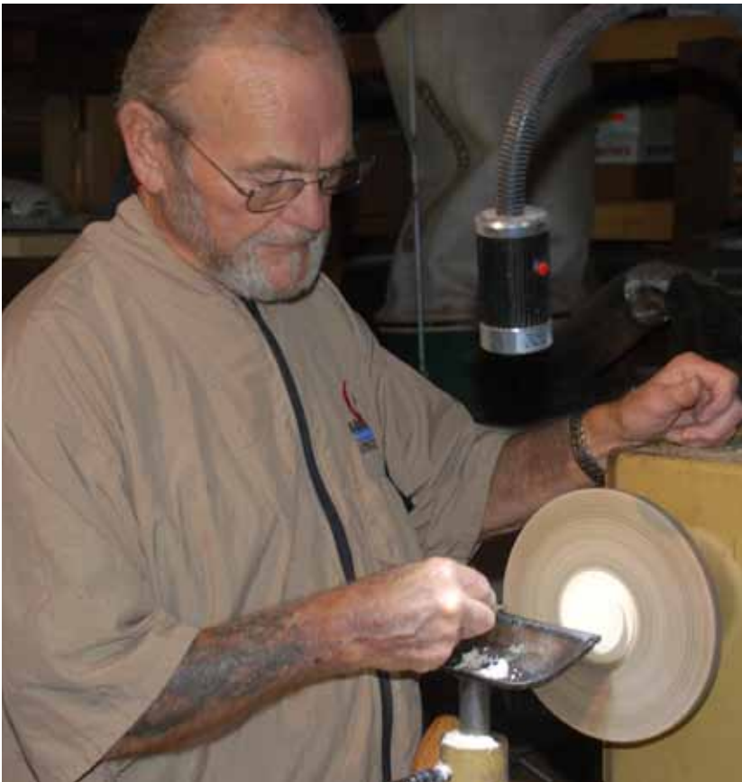
Rawson Beals burns the valleys between beads using heavy paper backed sandpaper.
