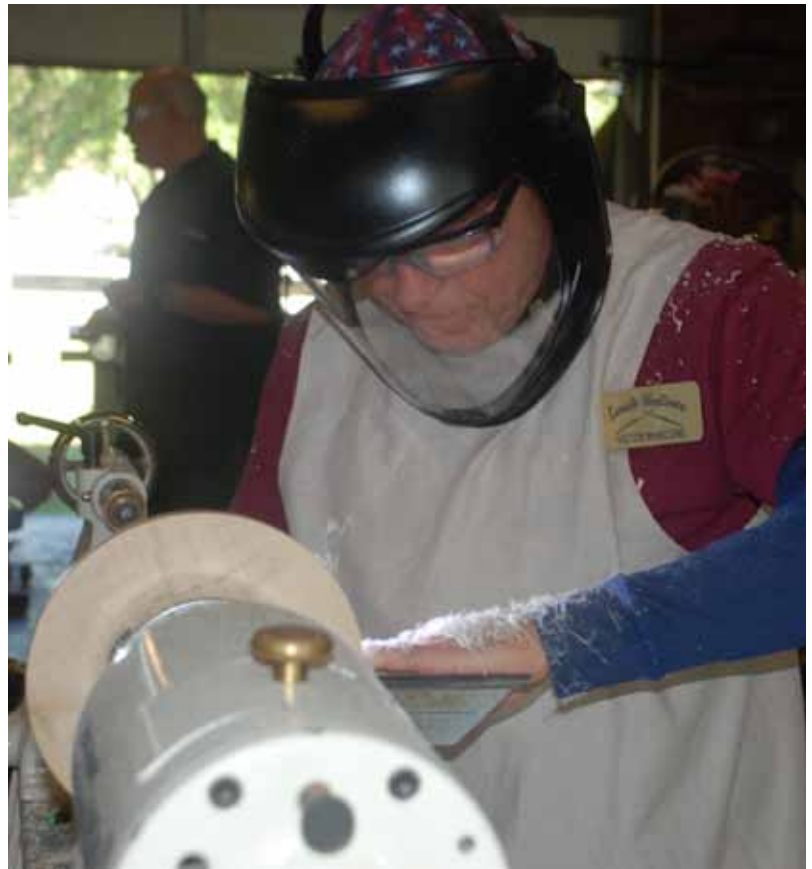
Victor Marccone using the d-way beading tools to score and cut the beads.
