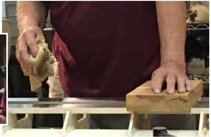
Polish with fine abrasive - run block of wood back and forth on bed.
