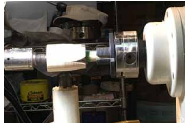
Mount the blank on a dowel and shape on lathe.
