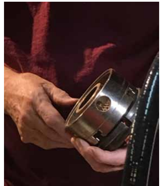
1200 grit sand paper removes dimple - pull paper under thumb.
