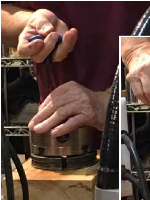
Clean under side of tool rest - oil with WD-40.
