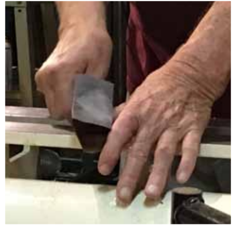
1200 grit sand paper removes dimple - pull paper under thumb.
