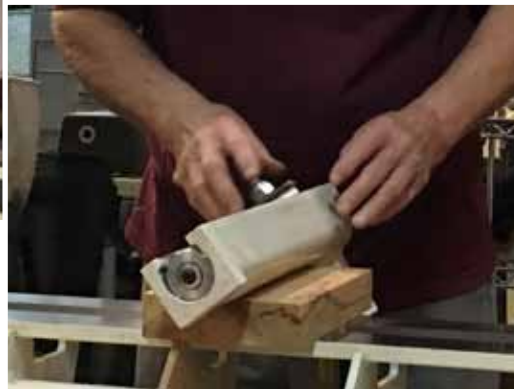
Clean under side of tool rest - oil with WD-40.
