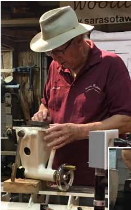
Clean under side of end stock - oil with WD-40.
