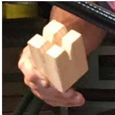
Cut curved "V"s in block.
