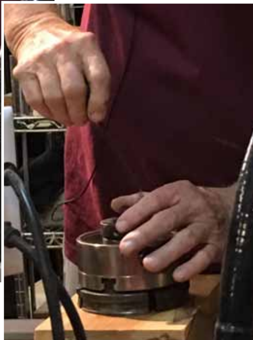
Disassemble chuck and clean thoroughly.
