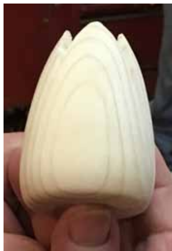
Cut curved "V"s in block.
