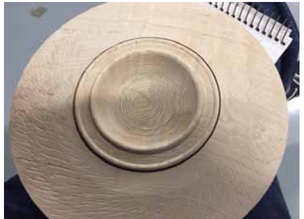
Wire brush spinning opposite direction to the wood can create an interesting texture effect on the wood's surface.
