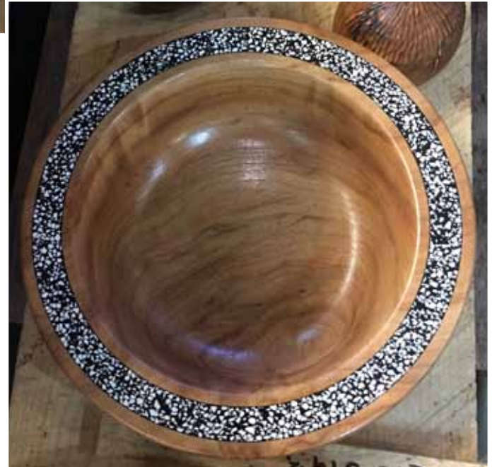
Hot glue gun beads along inner and outer edges of groove. Black inlay material, add white nuggets.
