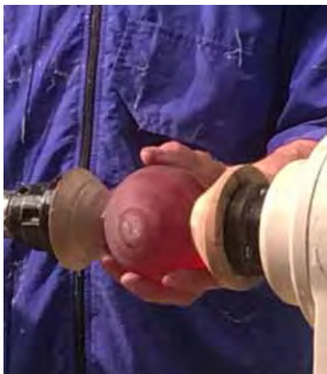
Russ places the sphere between two home made cup centers and carefully rounds with a negative rake scraper, turning the sphere 90° or 45° until round.
