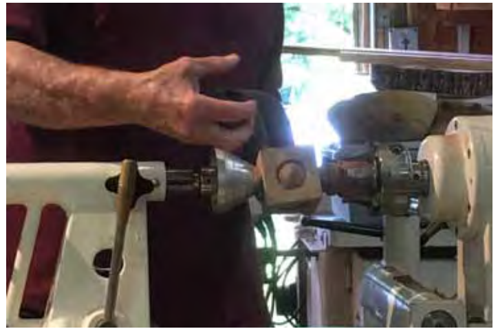
He sands the sphere with plumbers sand paper, running the lathe slowly.
