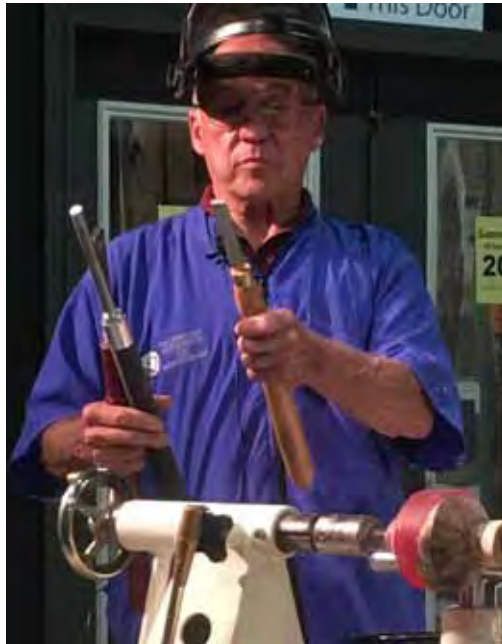
Russ uses a spindle gouge, a bowl gouge and a negative rake scraper to round the sphere. It is not good to breathe in the resin shavings.
