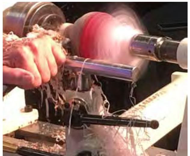
Russ uses a spindle gouge, a bowl gouge and a negative rake scraper to round the sphere. It is not good to breathe in the resin shavings.
