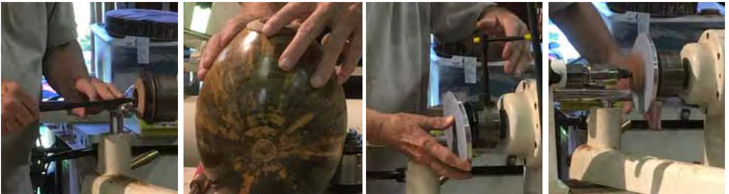
Using a Simon Hope Aluminum face plate with a velcro sanding disk, he rounds out a walnut block with a gouge. He flattens the front, rounds the sides and cuts to size for threading.
