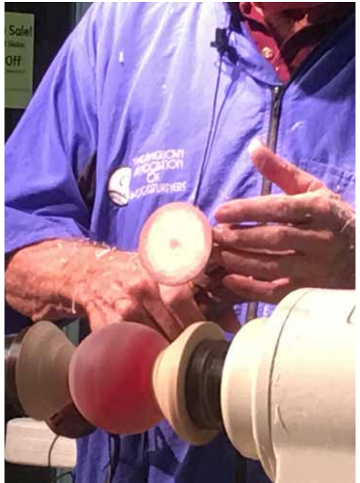
He then sands the sphere with low grits up to 400 and then wet sands from 600 – 1200 grit. again turning the sphere 90° or 45° until smooth.
