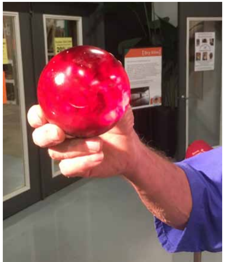
He then sands the sphere with low grits up to 400 and then wet sands from 600 – 1200 grit. again turning the sphere 90° or 45° until smooth.
