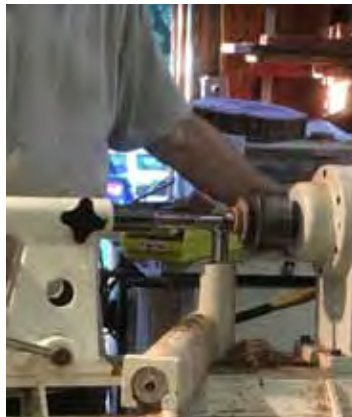
Use a parting tool, burr up. Sand and apply CA glue. Put wax on threads. Drill 1/4" hole for finial.
