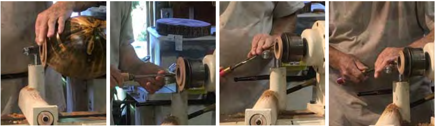
Franck fits a walnut top with cutted threads into the urn. He then gets rid of excess wood with a 3/8" bowl gouge, shaping an ogee curve. He cuts away the first thread and stiffens with CA glue.
