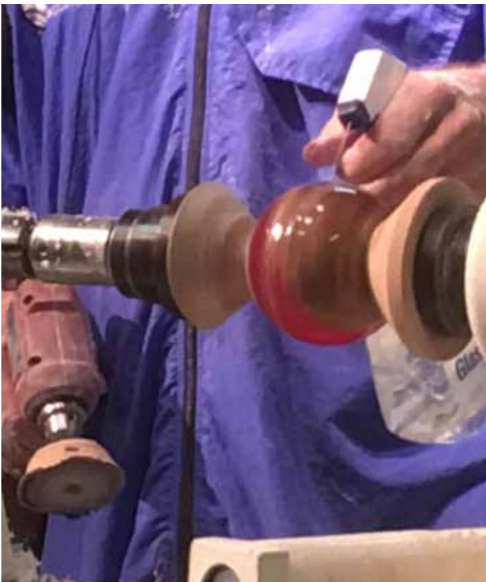
He then sands the sphere with low grits up to 400 and then wet sands from 600 – 1200 grit. again turning the sphere 90° or 45° until smooth.
