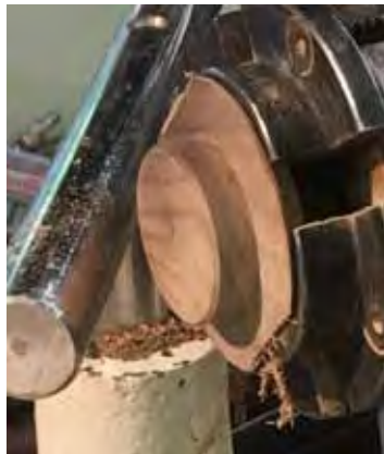
Use a parting tool, burr up. Sand and apply CA glue. Put wax on threads. Drill 1/4" hole for finial.
