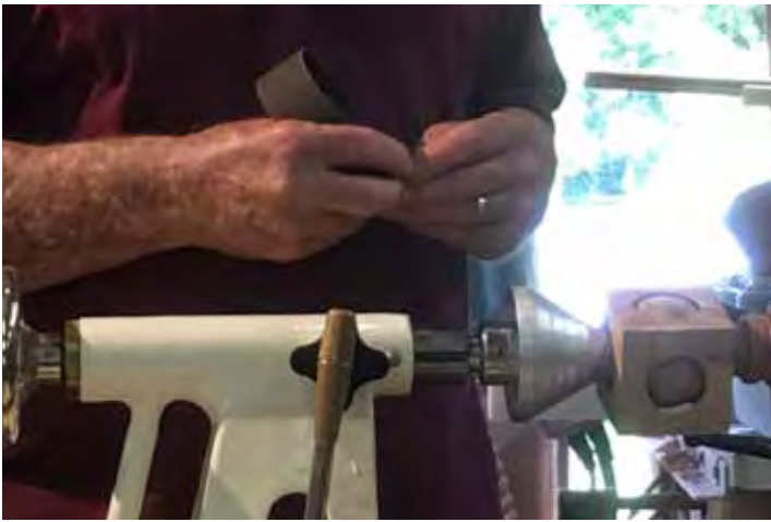
He sands the sphere with plumbers sand paper, running the lathe slowly.
