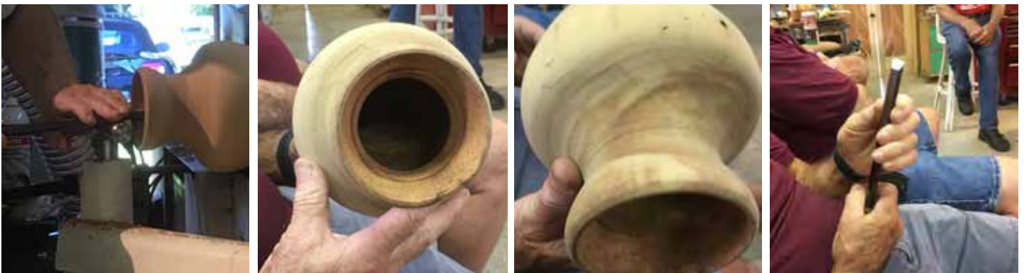
To remedy this he turns and adds a base for the piece. After cutting a tenon on the bottom of his Camphor vase with his Cindy Drozda scraper, he reverses and centers the piece in a chuck. He then gently squares the top, tilting the angle toward the mouth.
