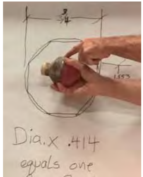
Russ begins with a hexagon, the diameter times .414 equaling one face of the octagon.
