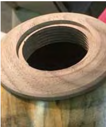
Use a parting tool, burr up. Sand and apply CA glue. Put wax on threads. Drill 1/4" hole for finial.
