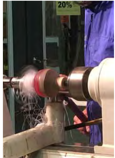
Russ uses a spindle gouge, a bowl gouge and a negative rake scraper to round the sphere. It is not good to breathe in the resin shavings.
