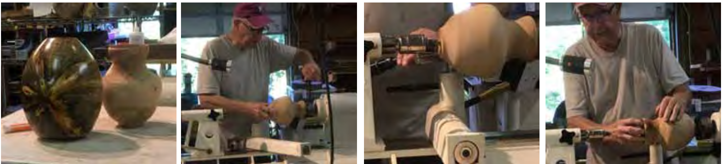
To remedy this he turns and adds a base for the piece. After cutting a tenon on the bottom of his Camphor vase with his Cindy Drozda scraper, he reverses and centers the piece in a chuck. He then gently squares the top, tilting the angle toward the mouth.
