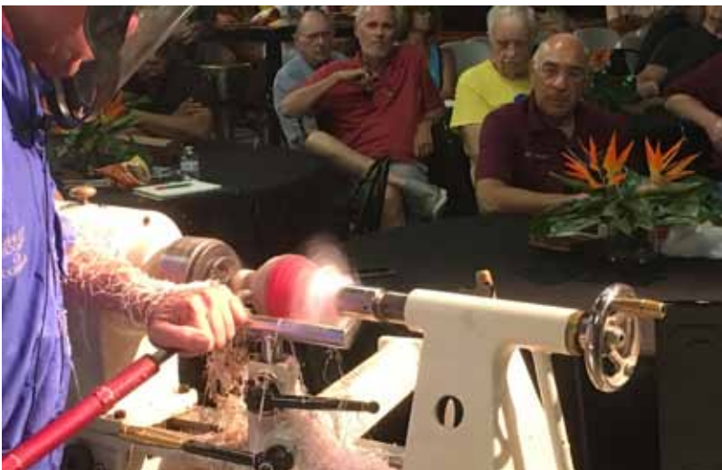
Russ uses a spindle gouge, a bowl gouge and a negative rake scraper to round the sphere. It is not good to breathe in the resin shavings.
