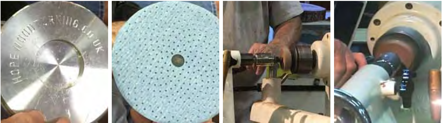
Using a Simon Hope Aluminum face plate with a velcro sanding disk, he rounds out a walnut block with a gouge. He flattens the front, rounds the sides and cuts to size for threading.
