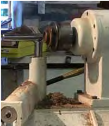
Use a parting tool, burr up. Sand and apply CA glue. Put wax on threads. Drill 1/4" hole for finial.
