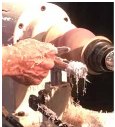
Russ places the sphere between two home made cup centers and carefully rounds with a negative rake scraper, turning the sphere 90° or 45° until round.
