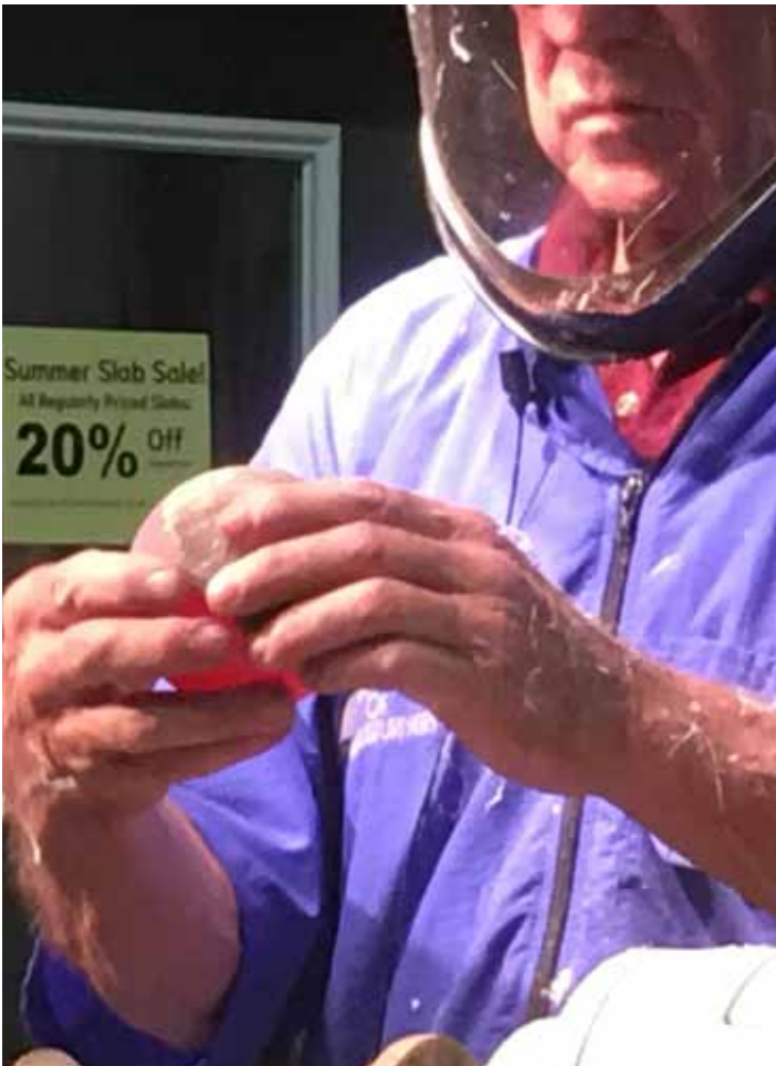
He then sands the sphere with low grits up to 400 and then wet sands from 600 – 1200 grit. again turning the sphere 90° or 45° until smooth.
