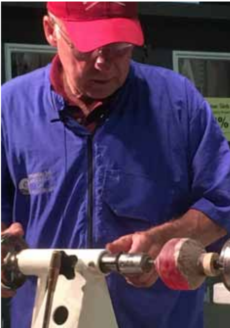
Russ uses a spindle gouge, a bowl gouge and a negative rake scraper to round the sphere. It is not good to breathe in the resin shavings.
