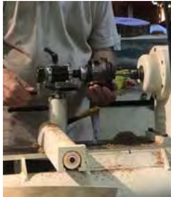
Use a parting tool, burr up. Sand and apply CA glue. Put wax on threads. Drill 1/4" hole for finial.
