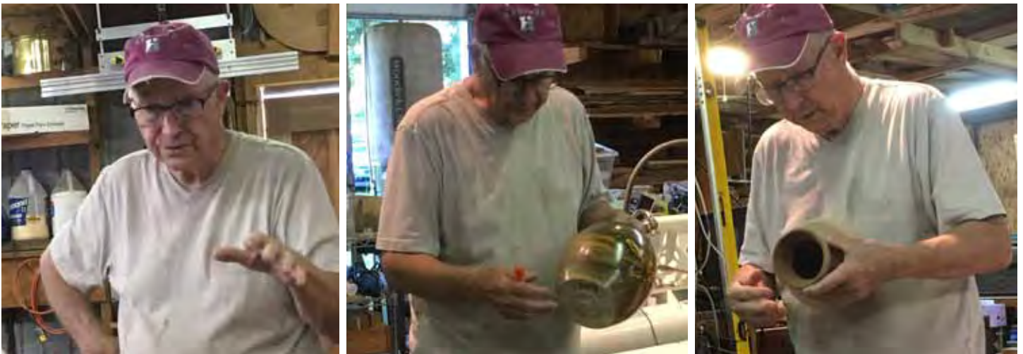
When turning urns Franck uses a face plate which leaves screw holes in the bottom.
