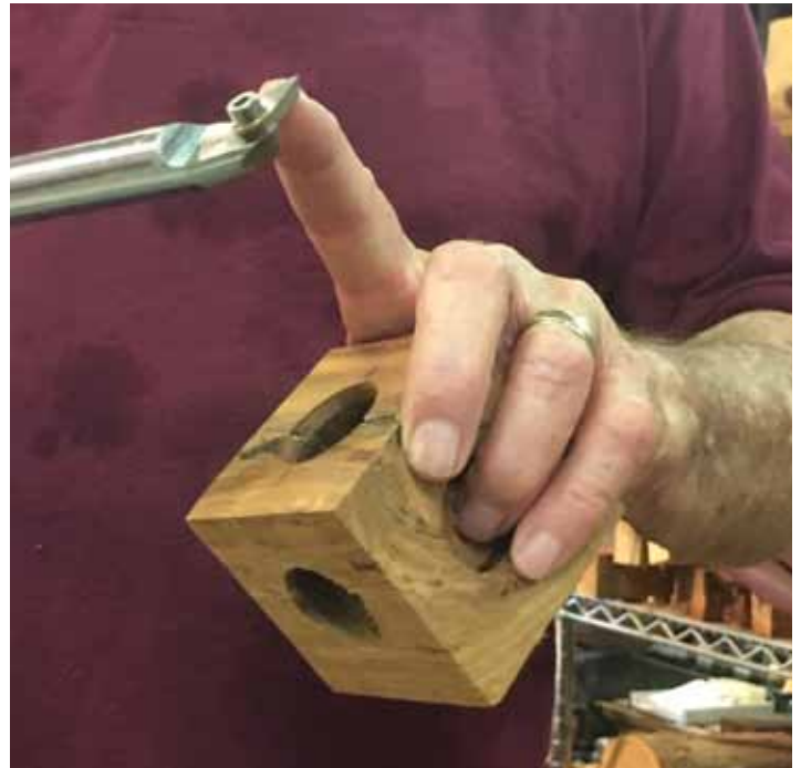
He drills with a Forstner Bit and carves with a modified Hope Hollowing tool.
