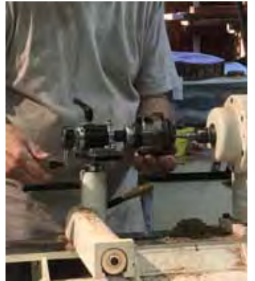
Use a parting tool, burr up. Sand and apply CA glue. Put wax on threads. Drill 1/4" hole for finial.
