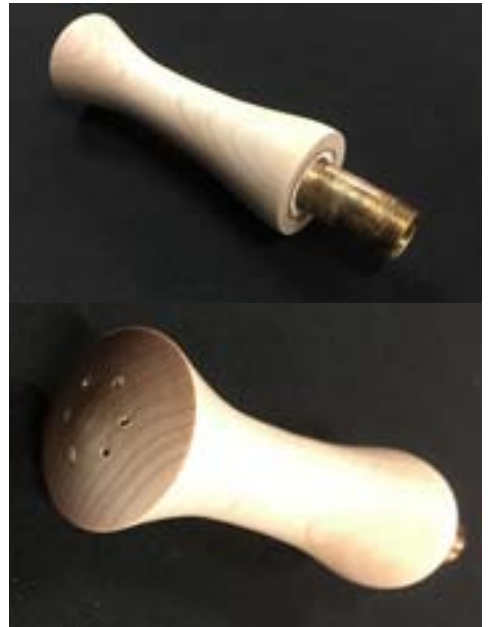
Ron removes the top with a spindle gouge and sands 120-400 grit with his home-made sander.
