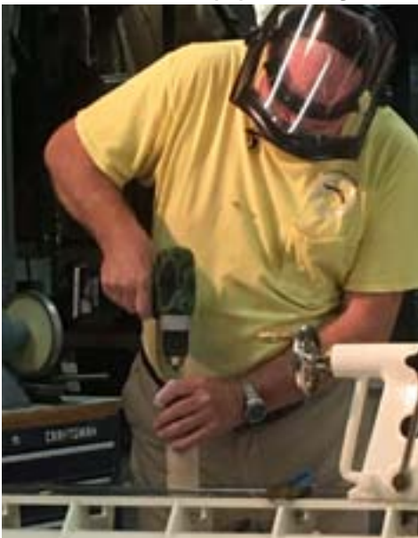
He then marks the shaker bottom, middle and top, using this metal template.
