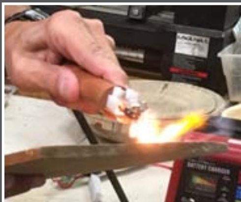
David Senecal's modified battery charger pyrography wood burning machine.
