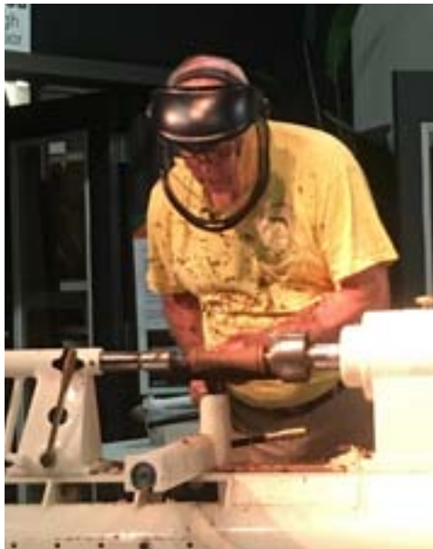
Ron applies 3408 with paper towel and sands with 600 grit paper to remove paper towel ridges.
