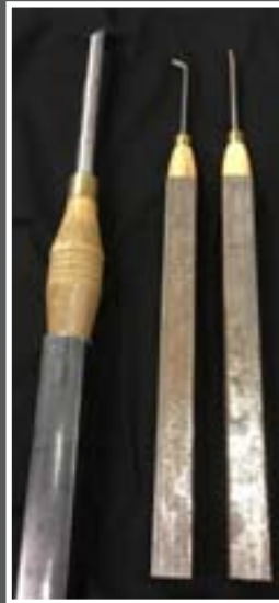
Pat added steel to tool handles to lengthen them.
