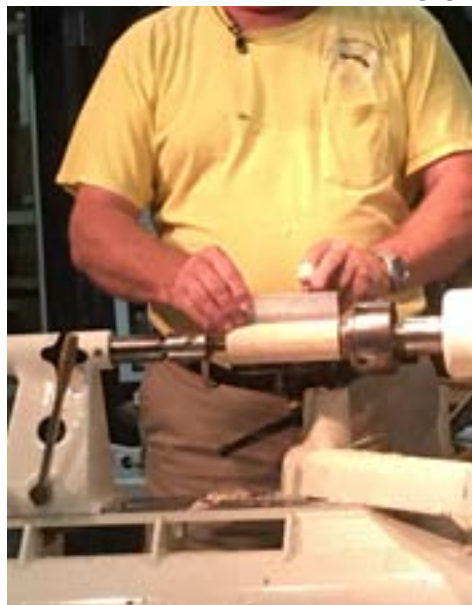
He then marks the shaker bottom, middle and top, using this metal template.
