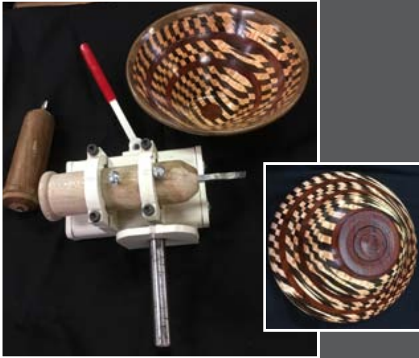
Charley Bell's modified ring cutter and 14 ring dippy bowl, assembled with Titebond III transparent glue and finished with seven coats Minwax Wipe-On-Poly, sanded between coats.
