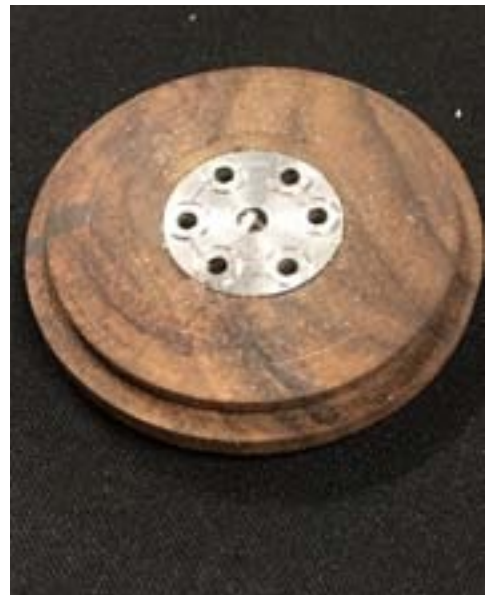
He removes the pipe fitting, inserts his washer/wooden drilling guide and drills 7/64" holes in top.
