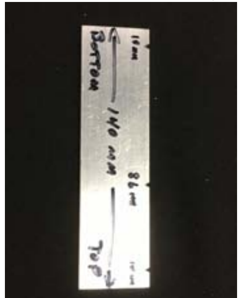
He then marks the shaker bottom, middle and top, using this metal template.
