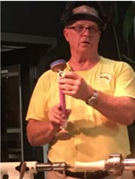
Ron removes the top with a spindle gouge and sands 120-400 grit with his home-made sander.
