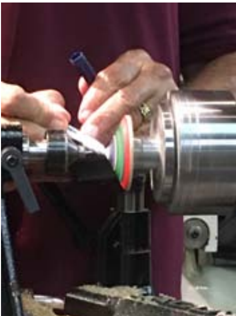
He adds texture with a dry wall screw and a round burr secured in a dowel. Color is added with markers. He finishes with 220 grit sand paper and applies carnuba wax.
