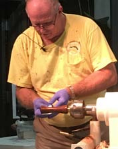
Ron applies 3408 with paper towel and sands with 600 grit paper to remove paper towel ridges.
