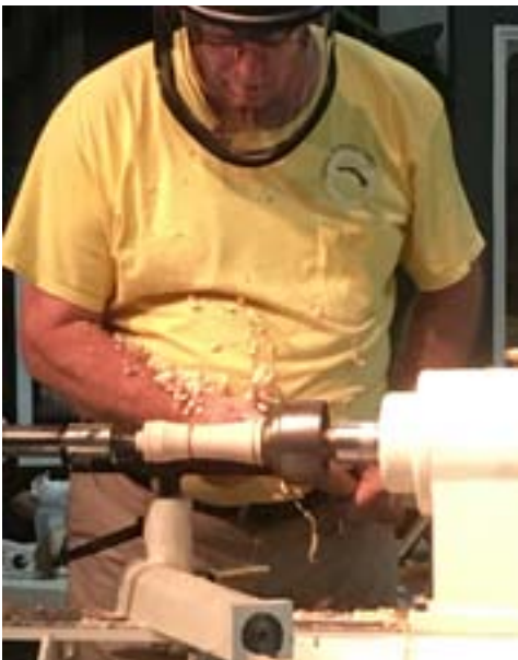
Ron removes the top with a spindle gouge and sands 120-400 grit with his home-made sander.
