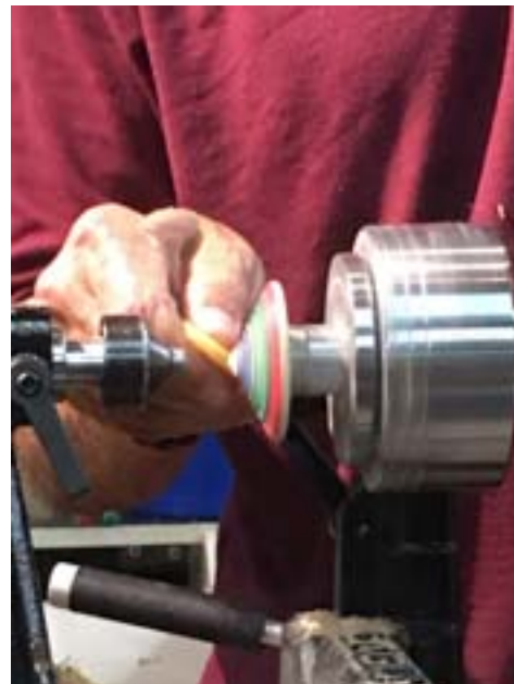
He adds texture with a dry wall screw and a round burr secured in a dowel. Color is added with markers. He finishes with 220 grit sand paper and applies carnuba wax.
