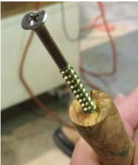
He adds texture with a dry wall screw and a round burr secured in a dowel. Color is added with markers. He finishes with 220 grit sand paper and applies carnuba wax.
