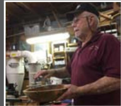
Pat used Wood Turners Finish on an older oil finished bowl and rosewood bracelets. He rubbed down with alcohol, applied 3 light coats, sanded with 320 grit and buffed.
