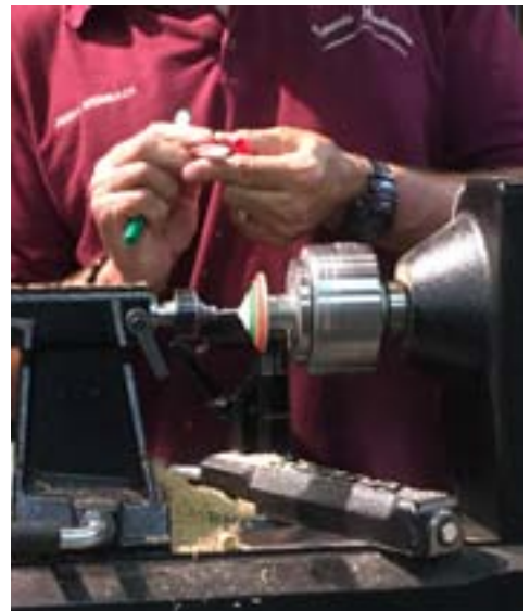
He adds texture with a dry wall screw and a round burr secured in a dowel. Color is added with markers. He finishes with 220 grit sand paper and applies carnuba wax.
