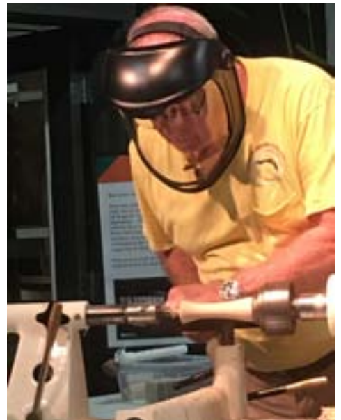
Ron removes the top with a spindle gouge and sands 120-400 grit with his home-made sander.
