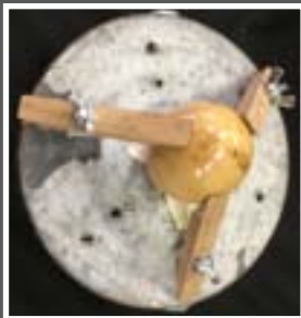
Pat Sullivan's Egg Ornament turned with Olive Wood from Bethlehem. A 3/8" hole drilled in top and then hollowed out. Face plate was made to hold egg on lathe.
