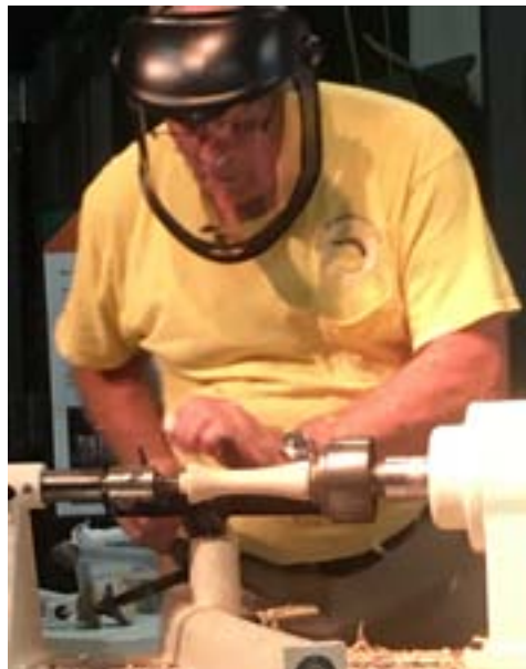
Ron removes the top with a spindle gouge and sands 120-400 grit with his home-made sander.
