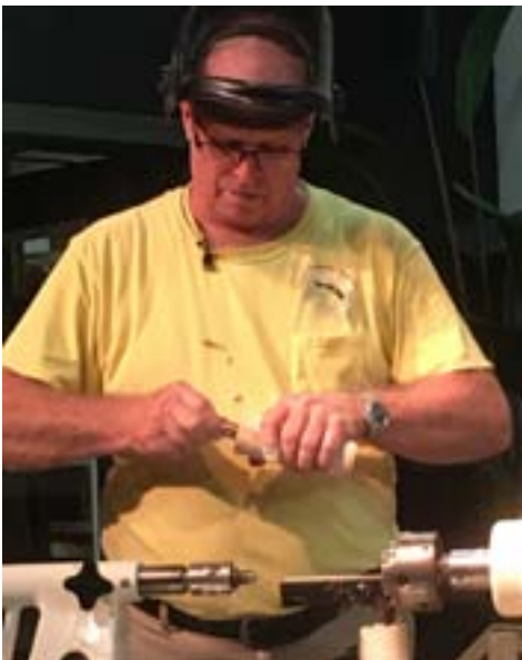
He removes the pipe fitting, inserts his washer/wooden drilling guide and drills 7/64" holes in top.
