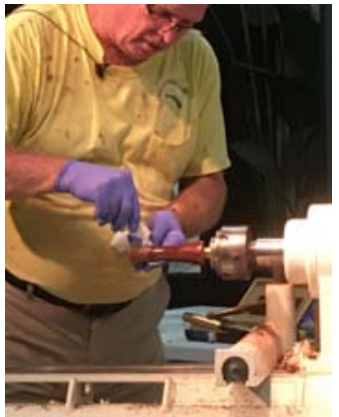
Ron applies 3408 with paper towel and sands with 600 grit paper to remove paper towel ridges.
