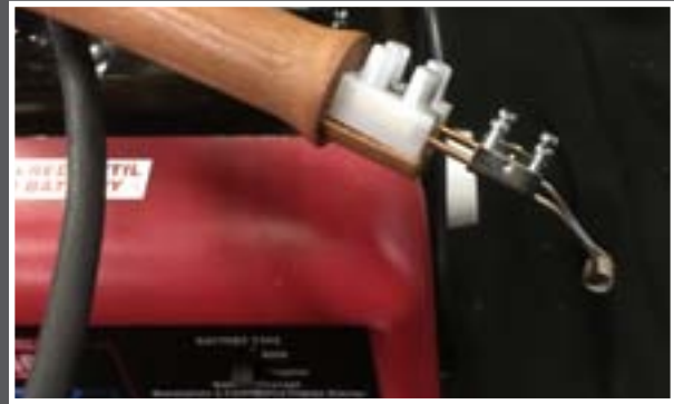
David Senecal's modified battery charger pyrography wood burning machine.
