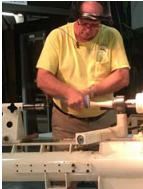
Ron removes the top with a spindle gouge and sands 120-400 grit with his home-made sander.
