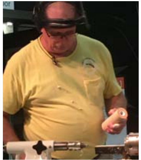
Ron cuts the plastic tube in half and then mixes epoxy and glue the tube into the wood.
