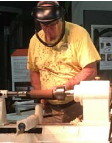
Ron applies 3408 with paper towel and sands with 600 grit paper to remove paper towel ridges.
