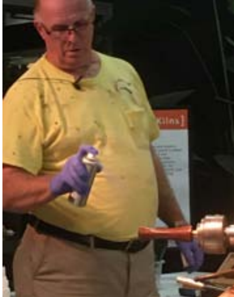
Ron applies 3408 with paper towel and sands with 600 grit paper to remove paper towel ridges.
