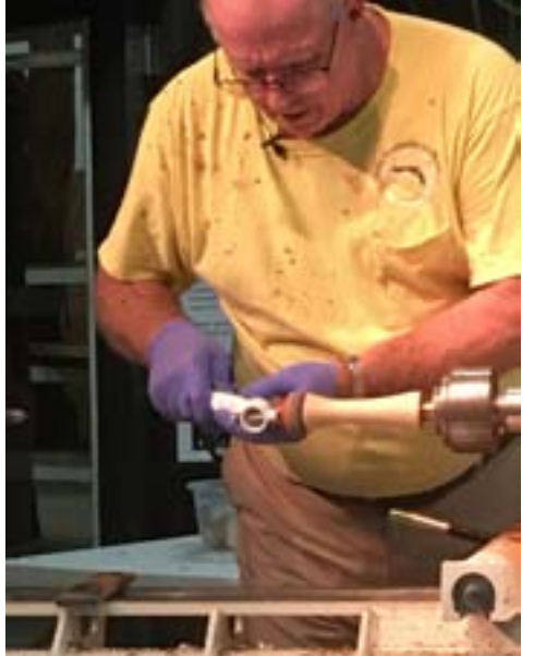
Ron applies 3408 with paper towel and sands with 600 grit paper to remove paper towel ridges.
